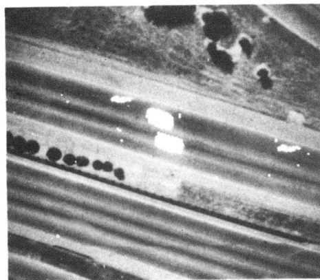
FIGURE 6(b) DETECTION OF ANOMALOUS AREAS ON THE ROAD SURFACE
