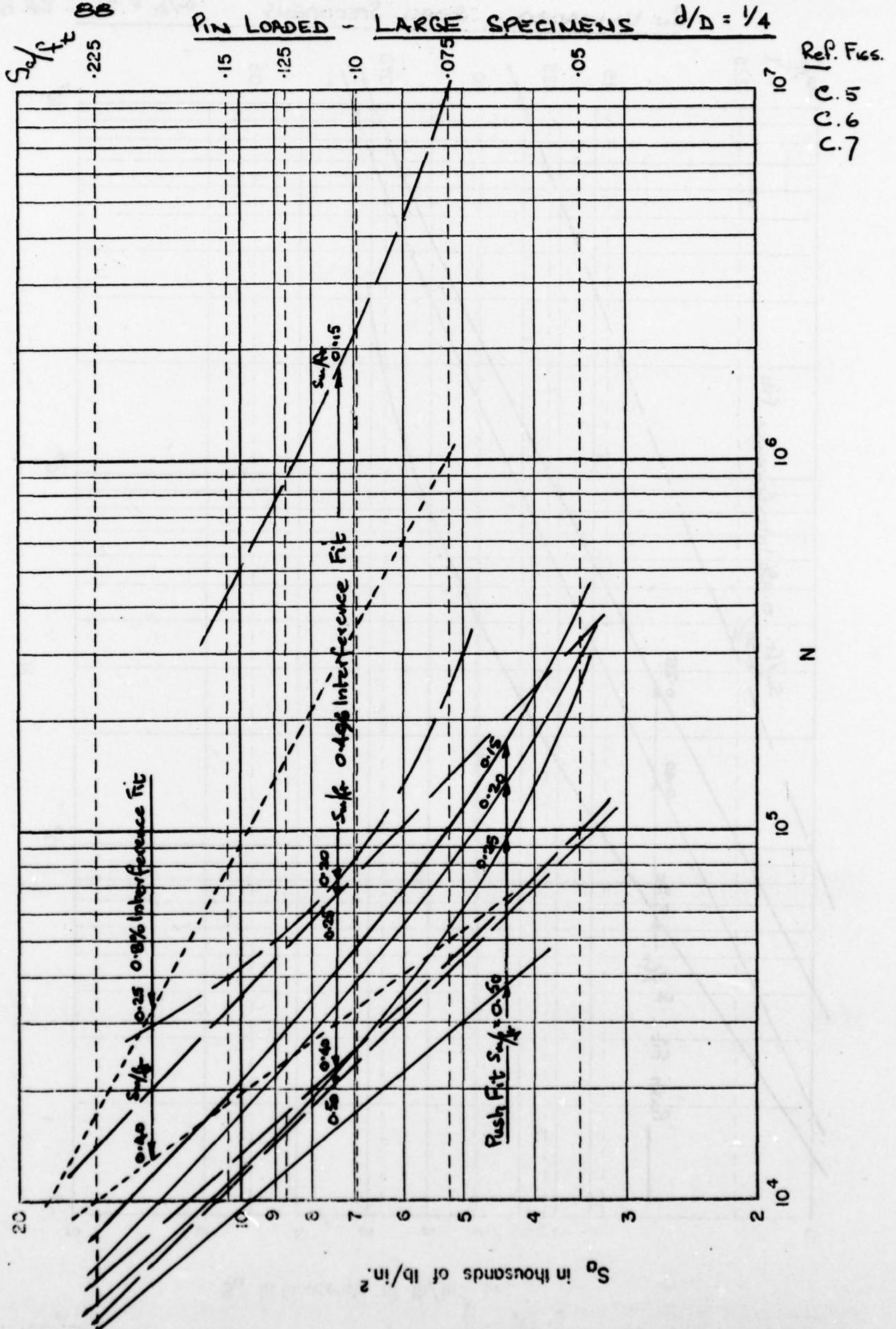
FIG. 4.28 COMPARISON BETWEEN PUSH FIT AND INTERFERENCE FIT PIN
