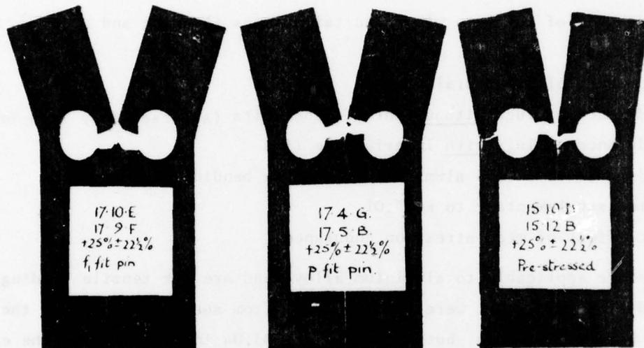
Comparison of failure origin between specimens tested at the same load but with different relationship between pin and hole.
