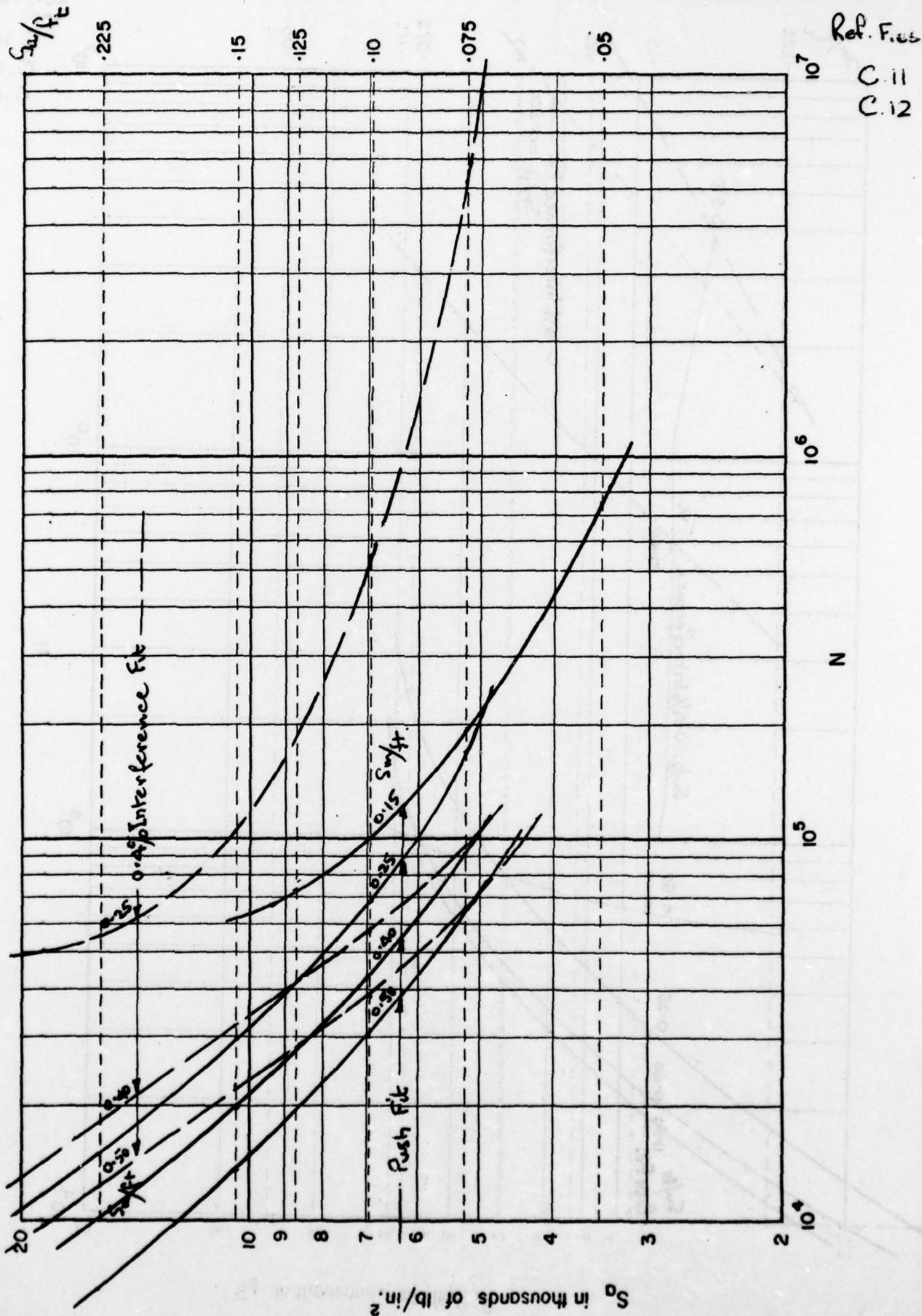
FIG. A-29 COMPARISON BETWEEN PUSH FIT & INTERFERENCE FIT PIN
