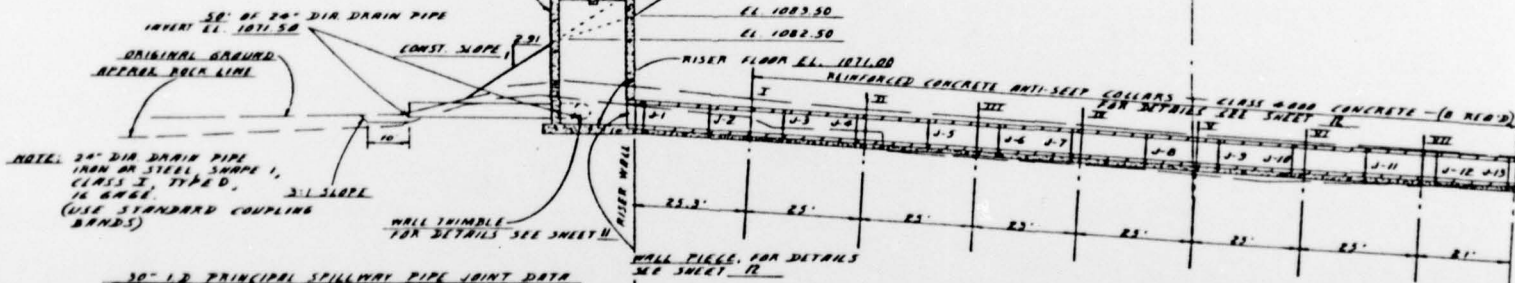
30" x 12" PRINCIPAL SPILLWAY PIPE JOINT DATA
