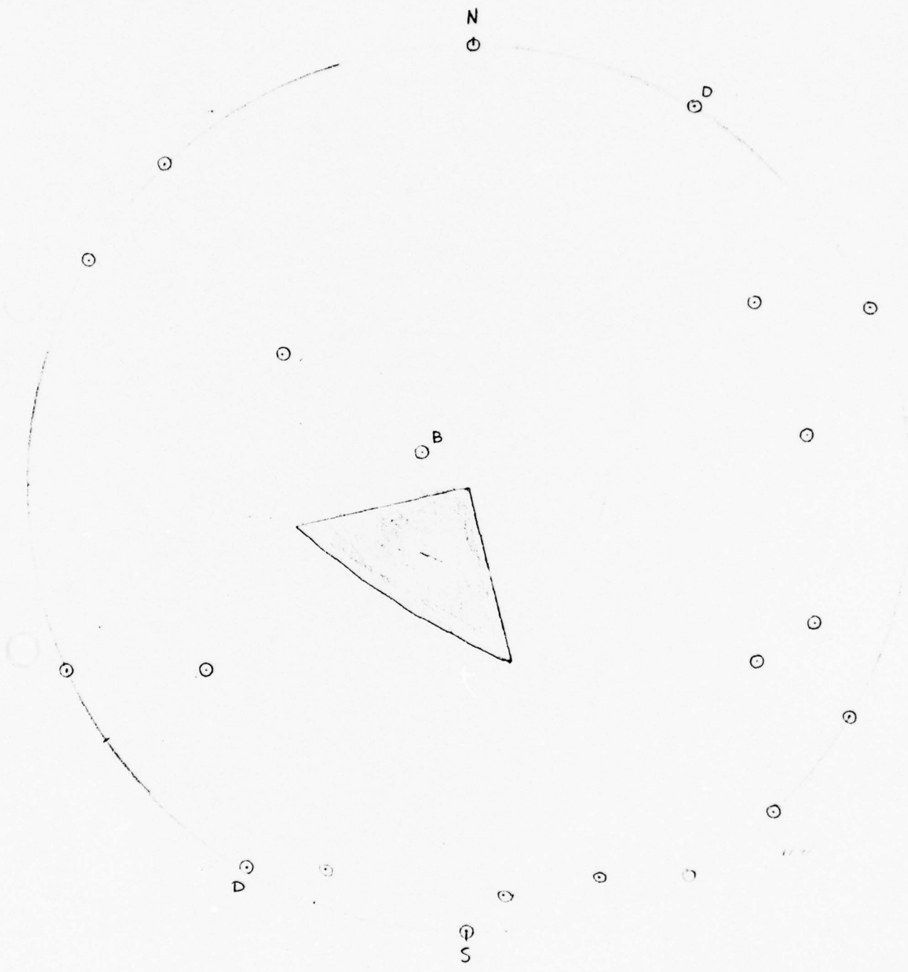
Figure 2. LAKE GORDON DAM Stereographic Plot of Poles to Joints (see text for explanation)
