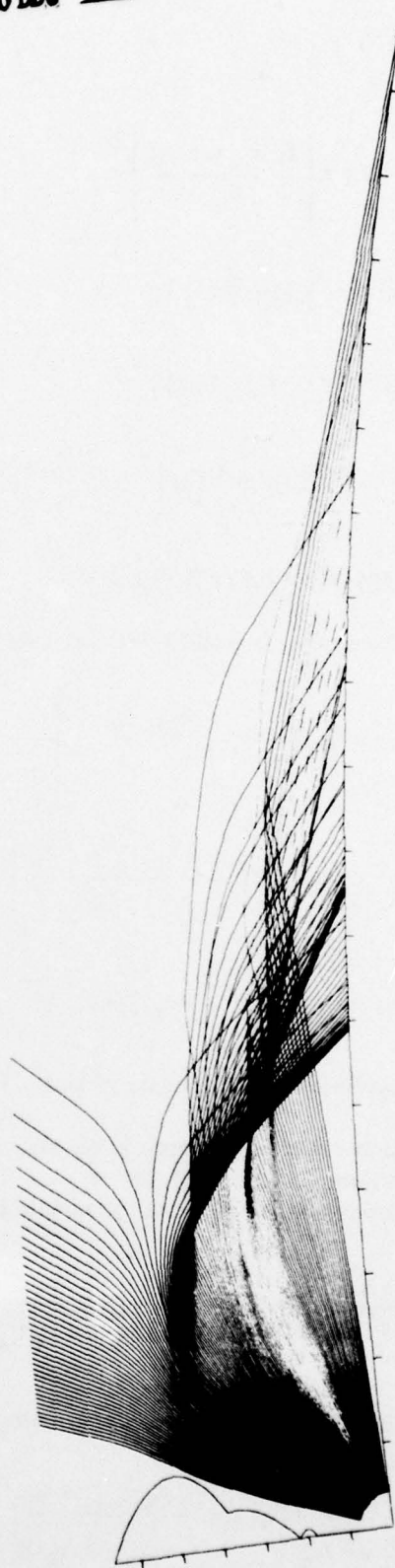
Figure 4. Ray fan in a three-layer ionosphere. The plasma frequency profile is displayed at the left side. The three layers produce three caustic surfaces, each having a "<" shape.
