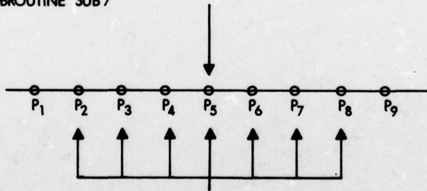
**Figure 9. Curve Smoothing Scheme (7-Point )**
