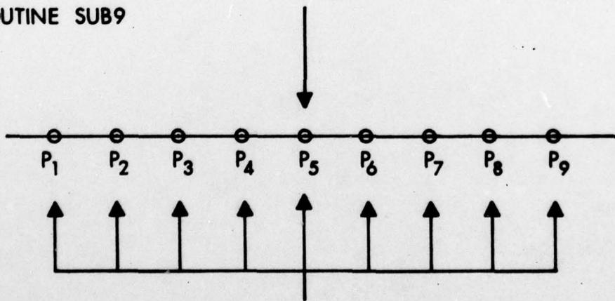
Figure 6. Curve Smoothing Scheme (9-Point)
