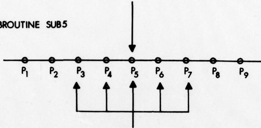
**Figure 8. Curve Smoothing Scheme (5- Point )**
