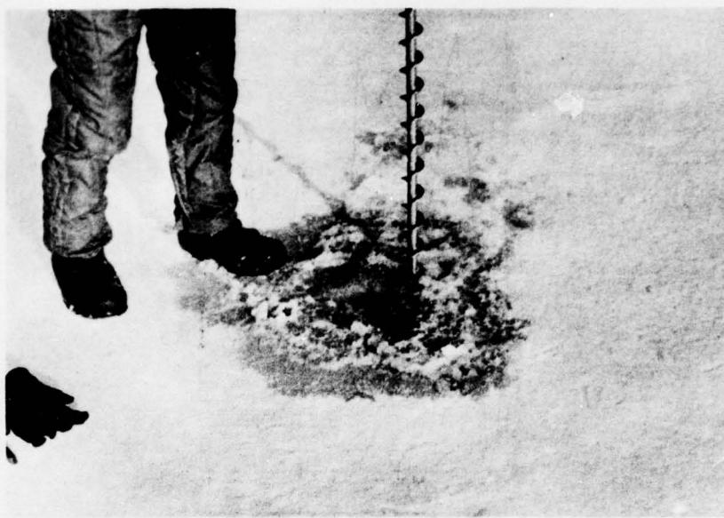
Figure 8. Typical ice auger hole with extracted frazil slush around perimeter.
