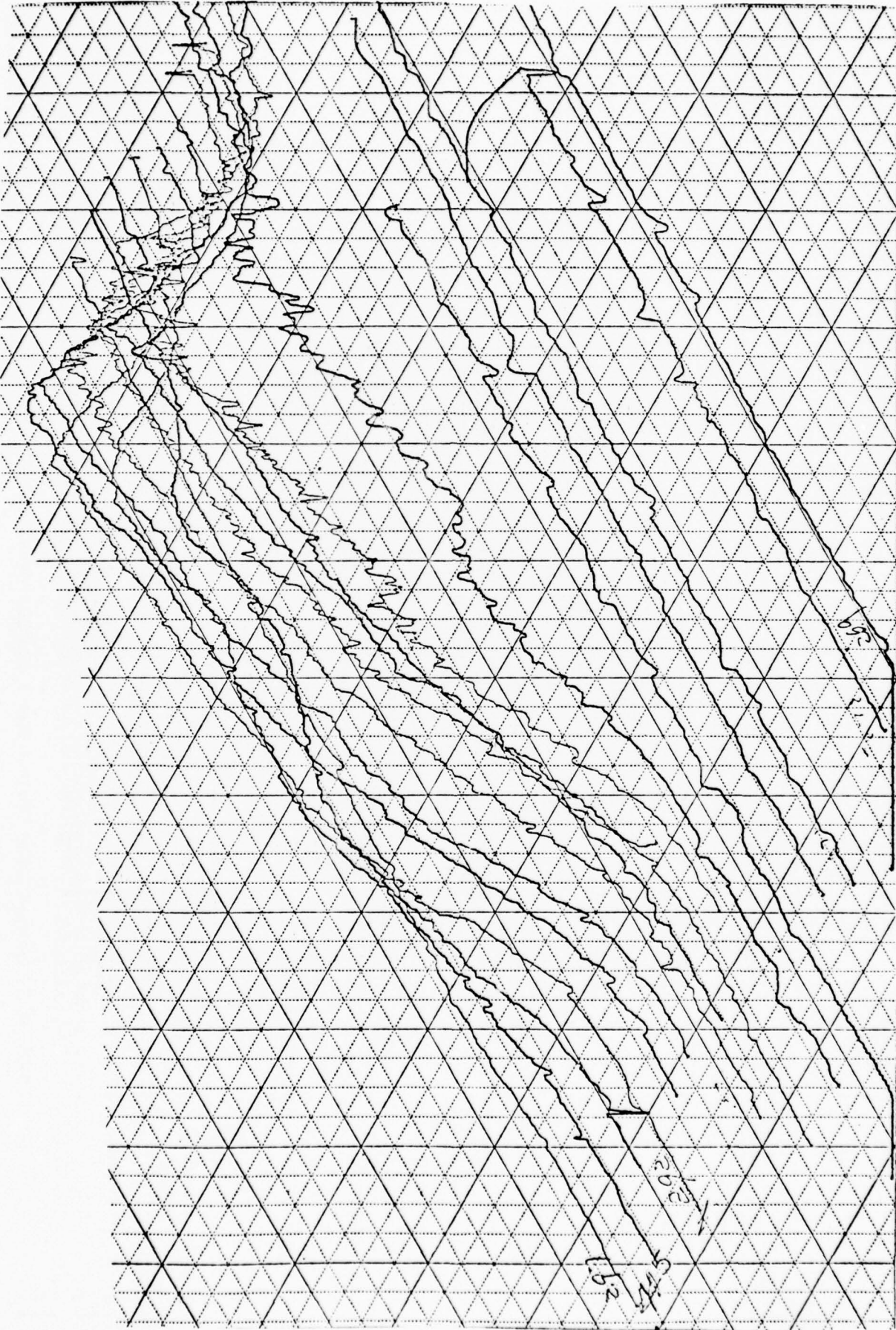
FIGURE 4.3 Pseudo - Three dimensional Responsivity Contour Map of Rockwell International Detector.
