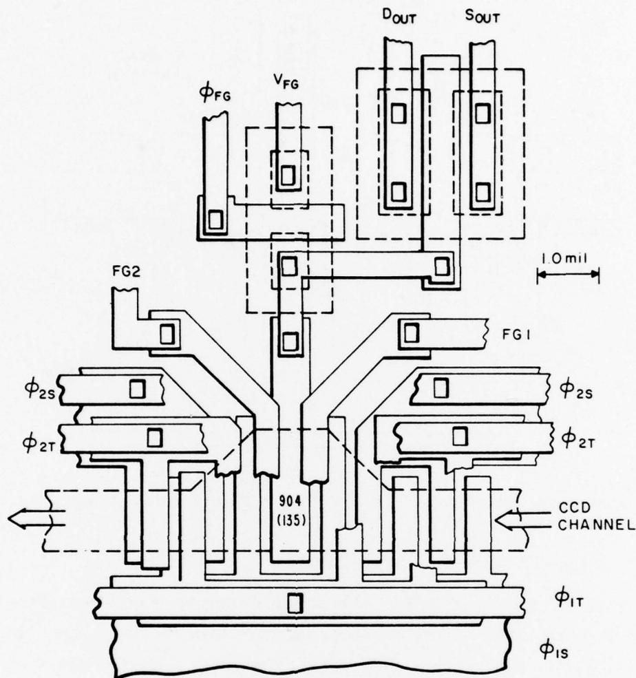
Figure 15. Layout of the floating-gate output stage.
