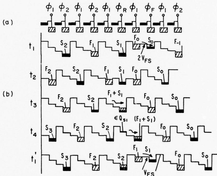
Figure 4. Low-loss CCD. (a) Charge-coupling structure. (b) Potential wells illustrating the operation.
