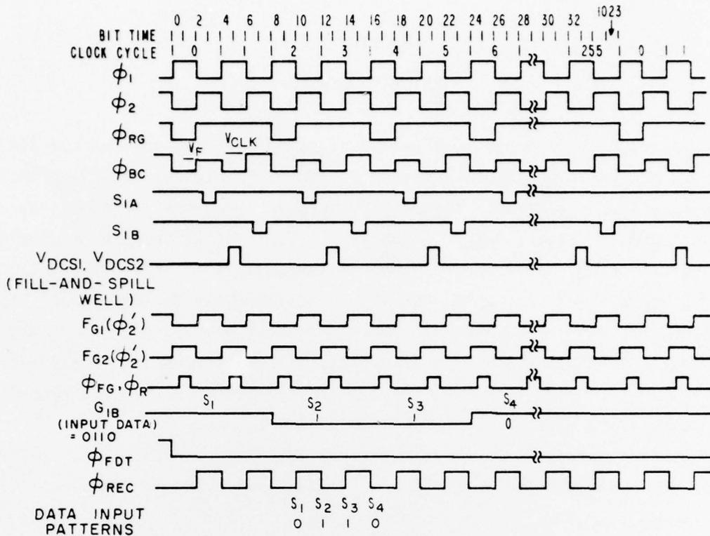
Figure 19. Detailed timing diagram of loop cycle 0 in Fig. 18.
