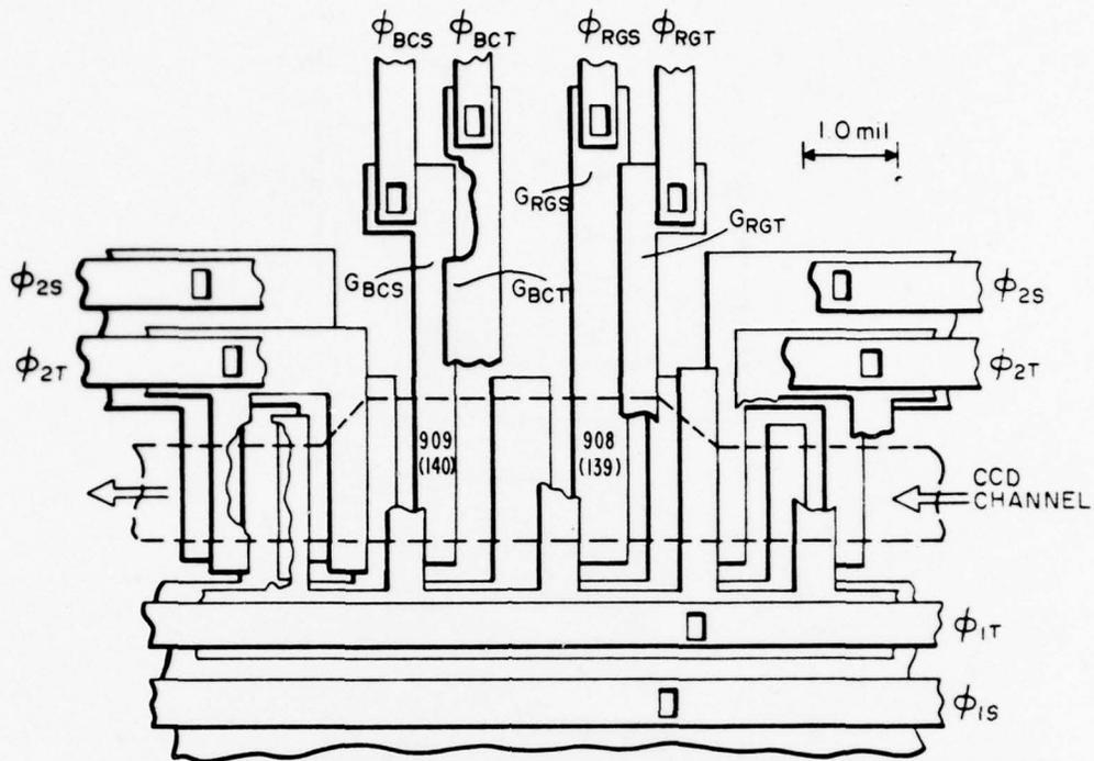
Figure 14. Layout of the low-loss signal-regeneration stage.
