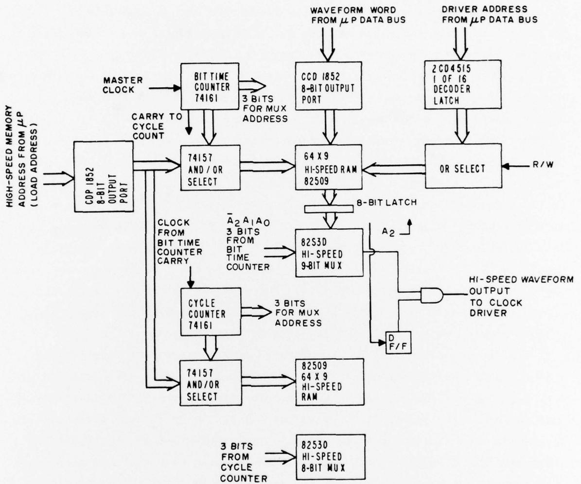
Figure 21. Auxiliary high-speed RAM for TC1230 test system.
