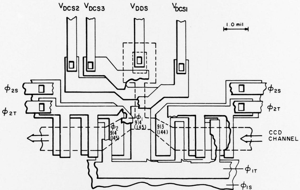
Figure 17. Layout of the dark-current subtraction stage.
