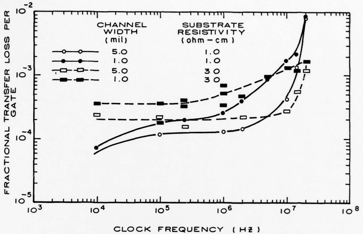
Figure 1. Transfer losses of surface-channel CCDs as function of clock frequency.
