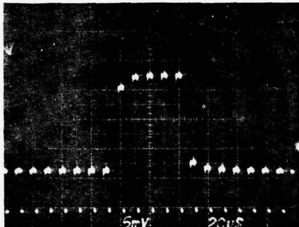
Figure 6. Output waveform of a 128-stage, two-phase SCCD operating in conventional CCD mode with an input signal in the form of five input samples. Vertical scale: 50 mV/div. Horizontal scale: 20  $\mu$ s/div.
