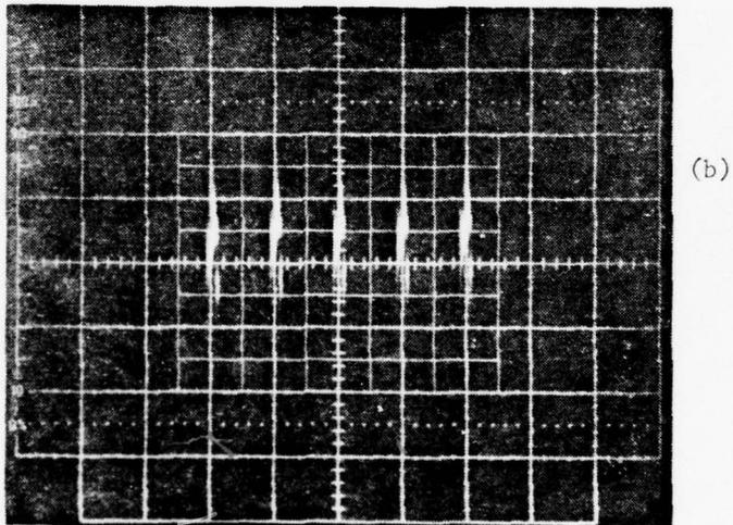
Figure 8. Output waveforms of 128-stage, two-phase SCCD operating with 20% bias charge in the signal stages and large (~100%) trailing bias charge in the alternate register stages. (a) Vertical scale: 50 mV/div. Horizontal scale: 20  $\mu$ s/div. (b) Vertical scale: 5 mV/div. Horizontal scale: 20  $\mu$ s/div.
