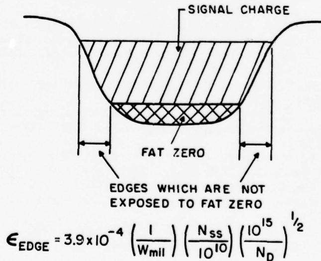
Figure 2. Edge-effect model for surface-channel CCD.
