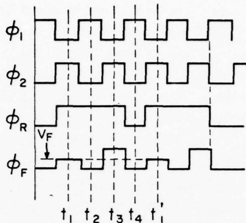
Figure 5. Clock waveforms for operation of the low-loss CCD shown in Fig. 4.
