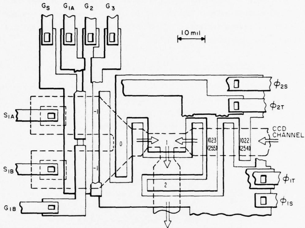
Figure 13. Layout of parallel inputs and merged input junction.
