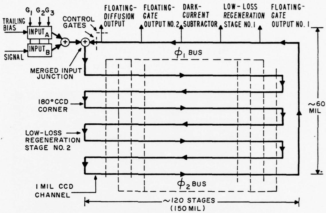
Figure 11. Schematic of the layout of the 1024- (or 1023-) stage CCD loop.
