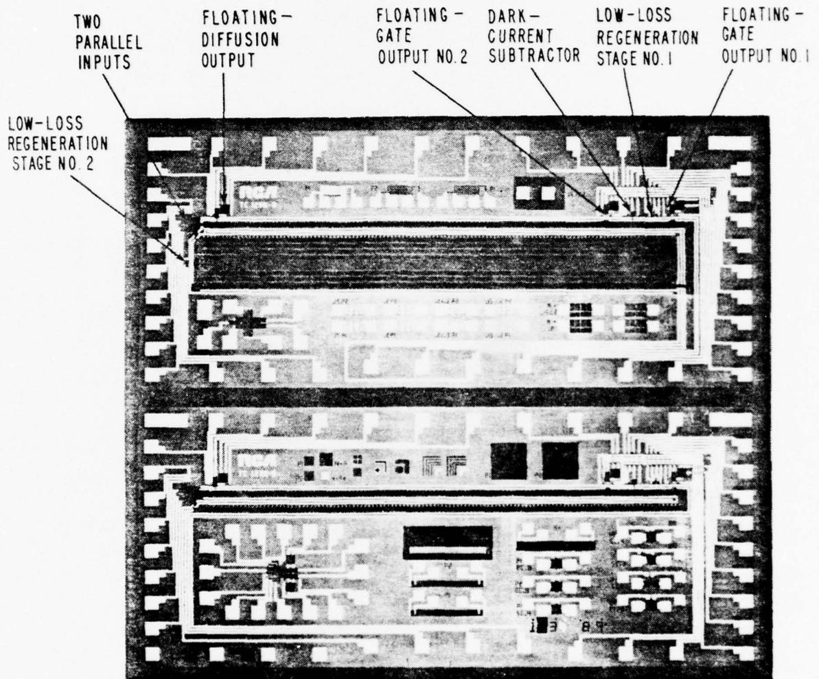
Figure 10. Photograph of the composite of the mask layers of the low-loss CCD test chip, TC1230.
