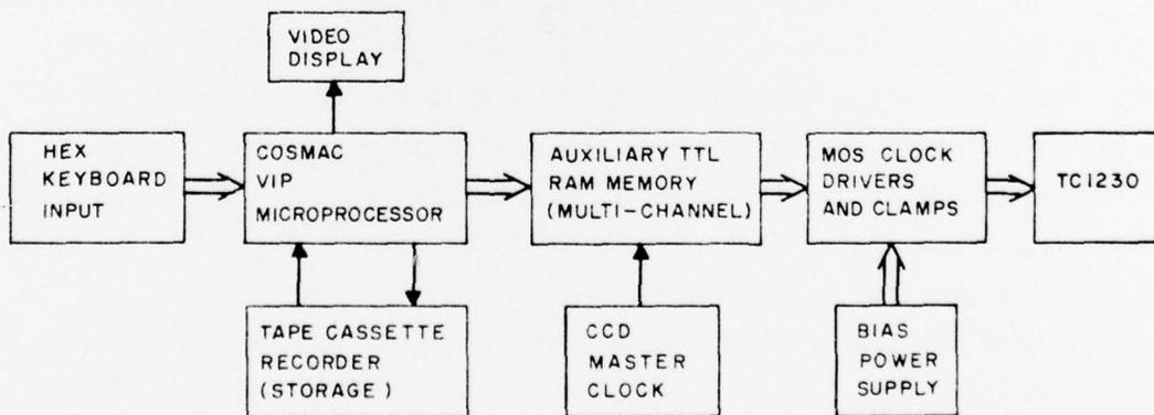
Figure 20. TC1230 test system.
