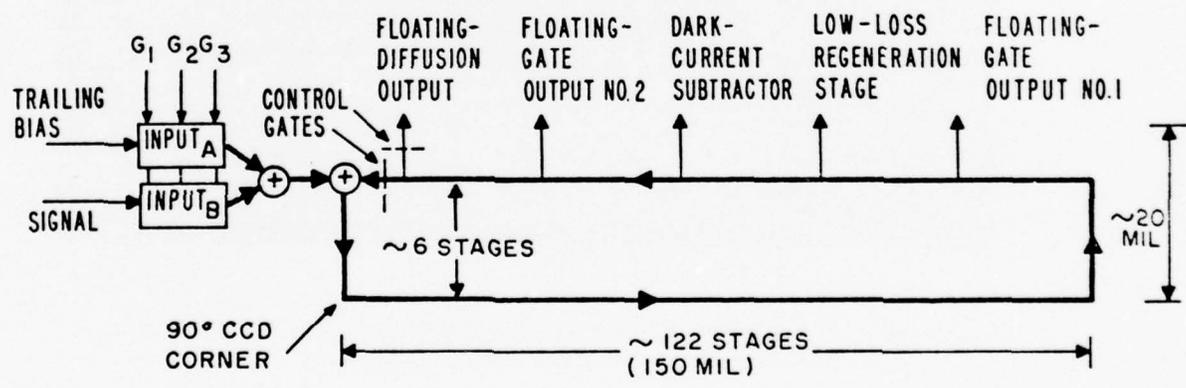
Figure 12. Schematic of the layout of the 256- (or 255-) stage CCD loop.
