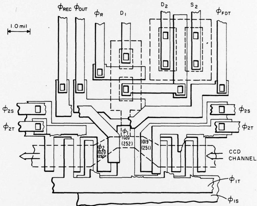
Figure 16. Layout of the floating-diffusion output stage.
