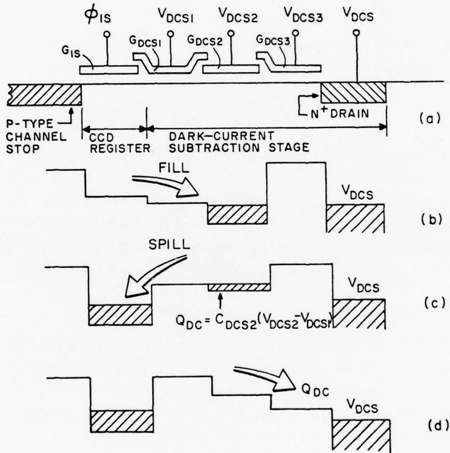
Figure 9. Construction and operation of the dark-current subtraction stage.
