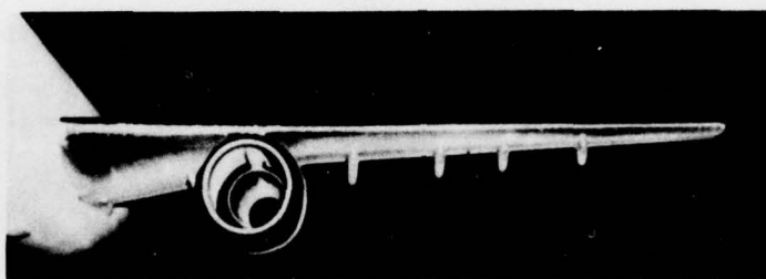
Fig. 19 — Similitude icing on a 1/12 scale model of Airbus.
