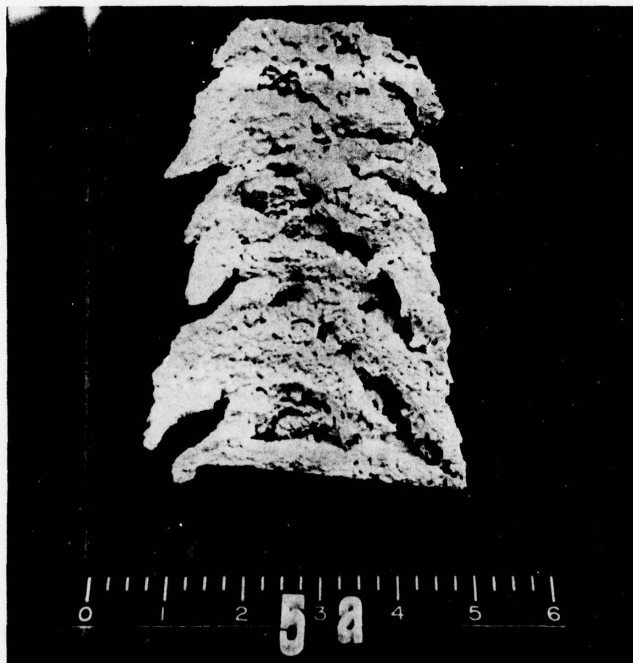
Figure 12—Sample Plaster Ice Cast
