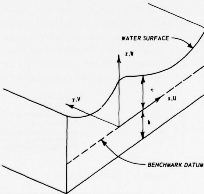
Figure 2. Coordinate system for problem formulation
