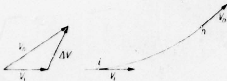
Figure 11. Change in the vector of velocity \Delta \vec{V} between velocity \vec{V}_n and the velocity at a current instant.
