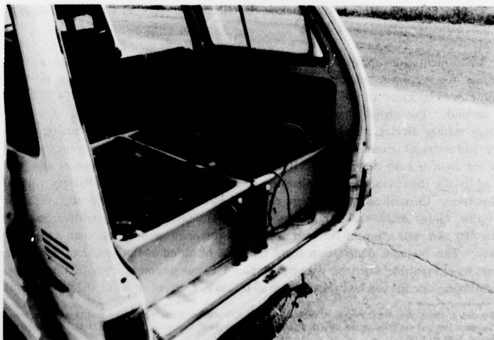
Figure 1B. Rear View Showing Batteries in Slide-Out Plastic Tubs.
