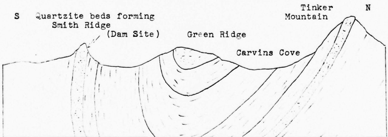
Figure 1. A generalized cross-section illustrating the ridge development and general structure at Carvins Cove. (Berkey 1924)
