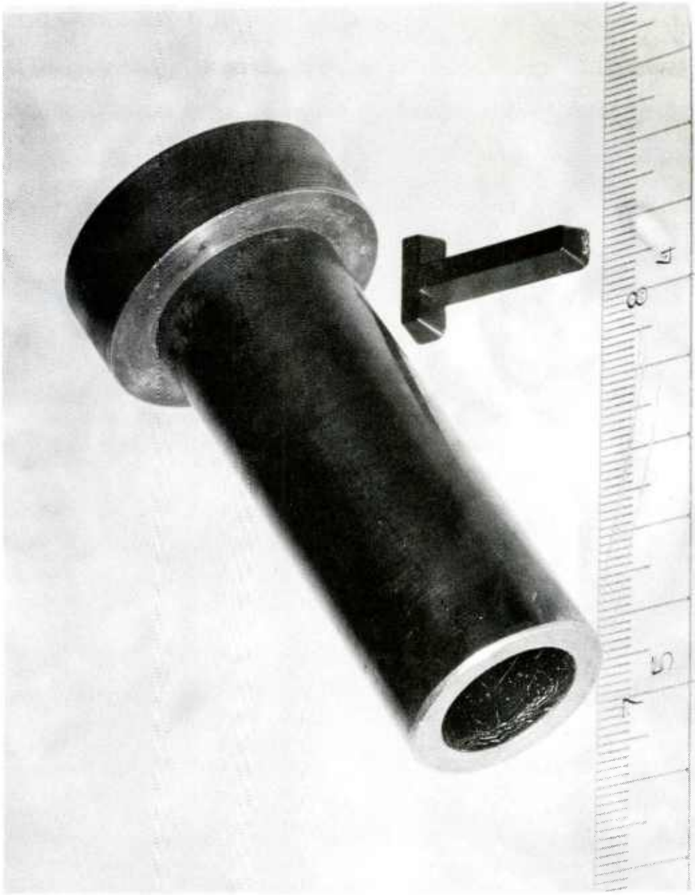
Figure 10. Typical example of damaged Teflon coating in agate exit ID surface.
