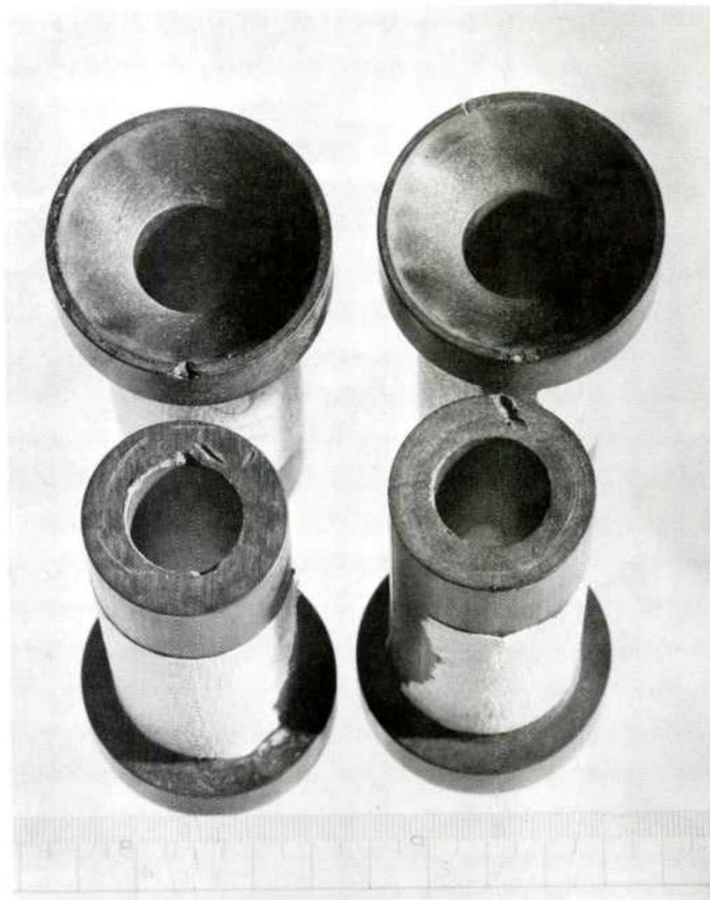
Figure 18. Typical graphite/Teflon/nylon agates with chips and dents in the approach angle and exit surfaces caused by production operations.
