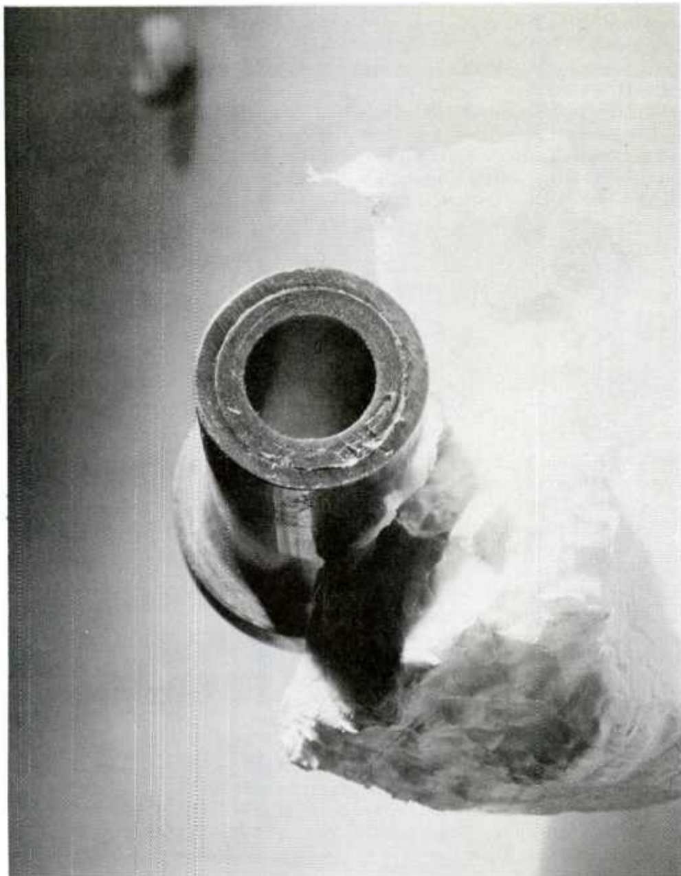
Figure 12. Delrin agate which has a damaged exit web and shows evidence of damage caused by the die agate removal tool.
