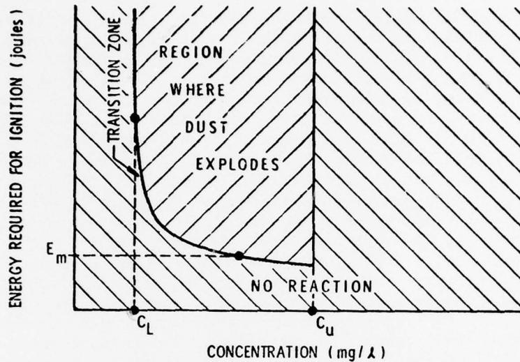
Figure 1-A. Typical Explosibility For A "Conventional" Flammable Dust
