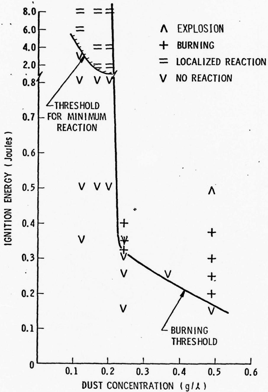
FIGURE 11. Dry M-1 Propellant Dust Explosibility
