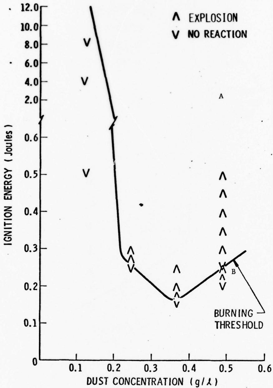
FIGURE 12. Dry M-1 Propellant Dust Explosibility
