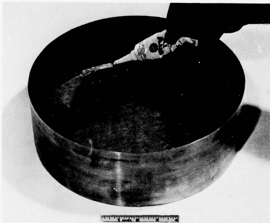
FIGURE 2.10 STEEL PLATE IN PLACE OVER THE LEAD SHOT, AND THE ASSEMBLY BEING SEALED WITH A SILICONE-RUBBER COMPOUND
