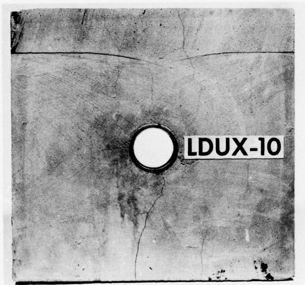
FIGURE 2.52 SECTIONED SPECIMEN FROM UNIAXIAL STRAIN TEST LDUX-10 ( P_V = 7 ksi, P_H = 4 ksi, \Delta D_V/D_V = 0.82\% , \Delta D_H/D_H = -0.77\% )
