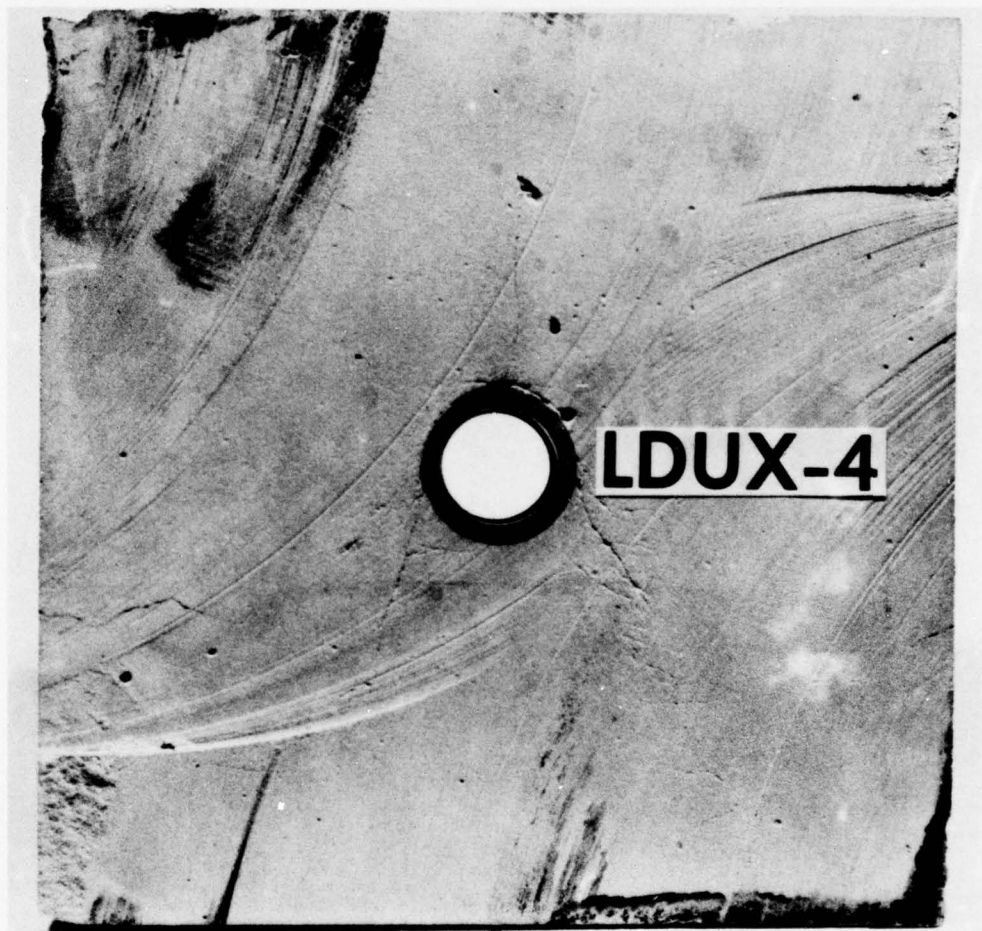
FIGURE 2.50 SECTIONED SPECIMEN FROM UNIAXIAL STRAIN TEST LDUX-4 ( P_V = 7 ksi, P_H = 4 ksi, \Delta D_V/D_V = 2.83\% , \Delta D_H/D_H = 1.23\% )
