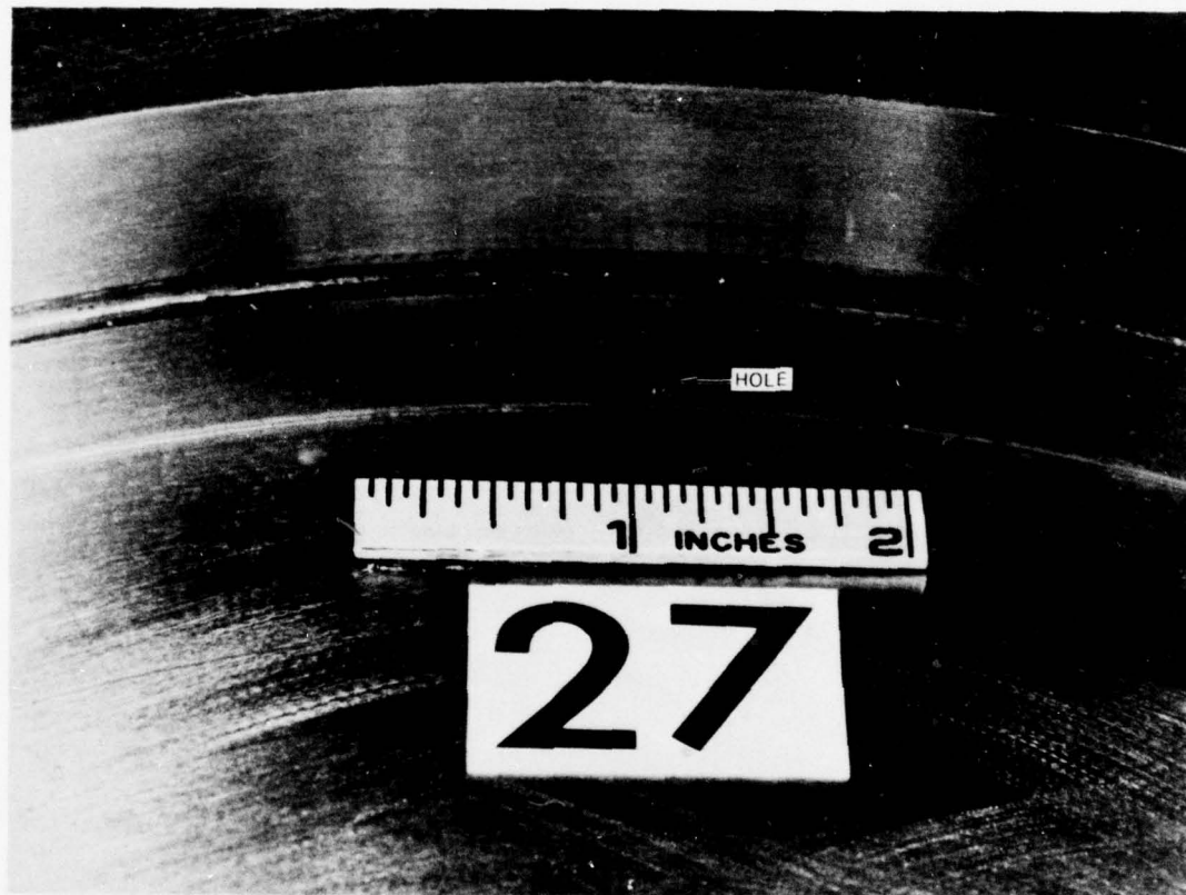
FIGURE 3.4 1/8-INCH DIAMETER PORT IN THE STATIC TOP VERTICAL/LATERAL SEAL PLATE USED TO APPLY VERTICAL LOADING PRESSURE
