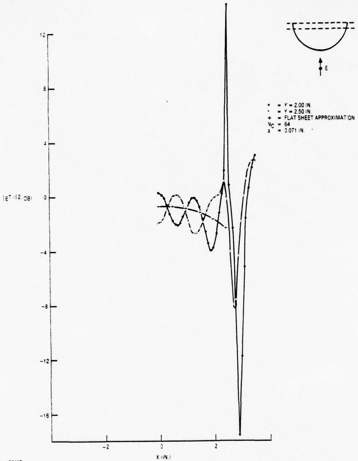
Figure 3-35. Power transmittance of dielectric hemi-cylinder for  $\theta_i = 90^\circ$ . Inner diameter 4.87 in.; thickness 0.125 in.; wavelength 1.259 in. Moment method calculations. Data are symmetric about  $X = 0$ .
