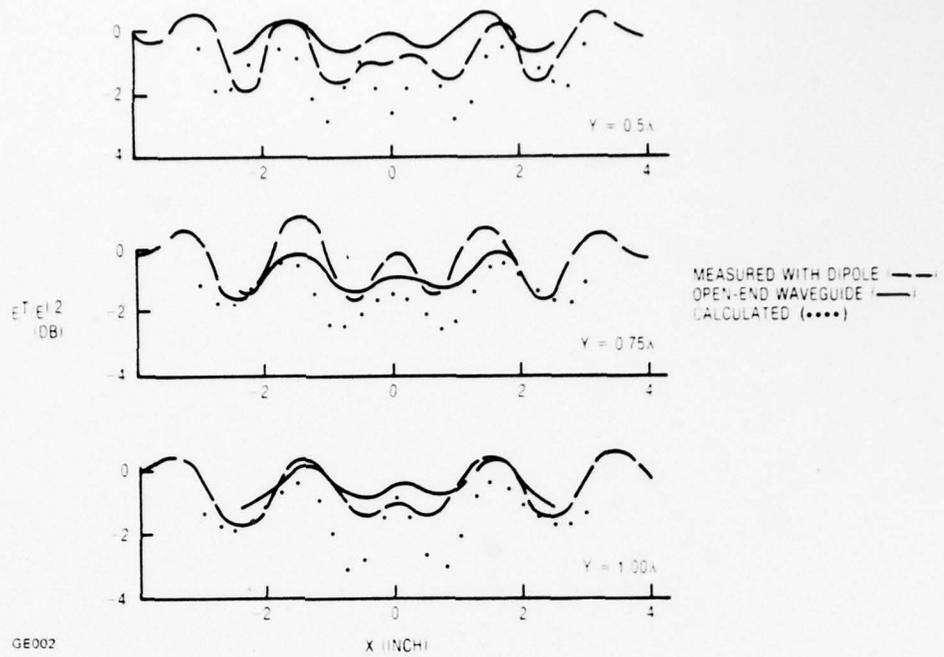
Figure 3-6. Power transmittance of  $0.24$  by  $4.0$  in. slab;  $\kappa = 2.6$ ;  $\phi_i = 0^\circ$ ;
