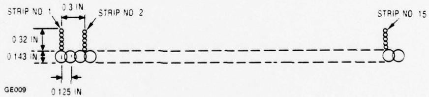
Figure 3-12. Array of 11 cylinders to represent 4.38 in. wide slab 0.125 in. thick with 15 strips.
