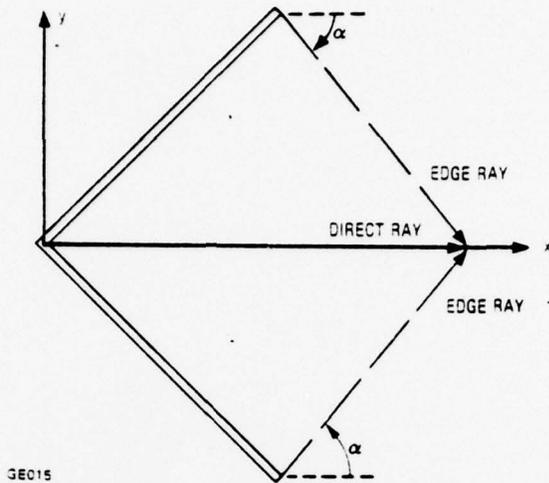
Figure 5-4. Hollow wedge; direct rays and edge diffracted rays shown for a point on symmetry plane
