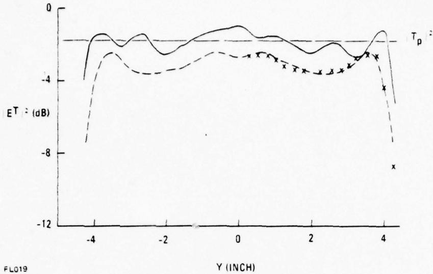
Figure 3-23. Intensity Behind Hollow Dielectric Wedge,  $\kappa = 2.6$ , With 10 in. x 18 in. Walls, Thicknesses 0.226 in. and 0.232 in. at  $\lambda = 1.259$  in. Measured with dipole probe (—). Calculated at  $x = 4.48$  in., for  $N = 81$  ( $^\circ$ ), for  $N = 83$  (x),  $a = 0.143$  in.,  $\rho = 0.25$  in.
