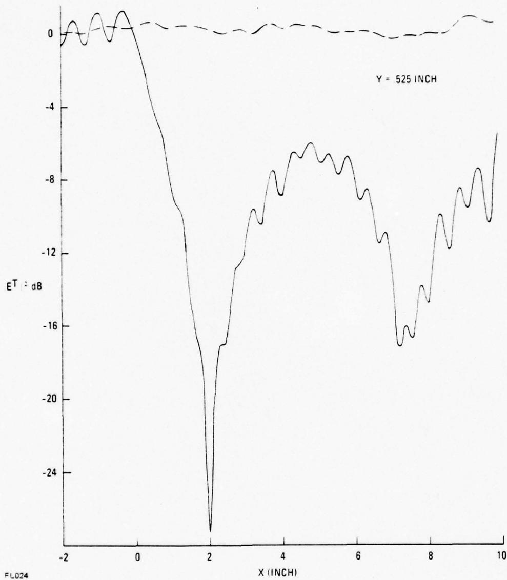
Figure 4-3. Measured Intensity Near Slab at Y = 0.525 in.
