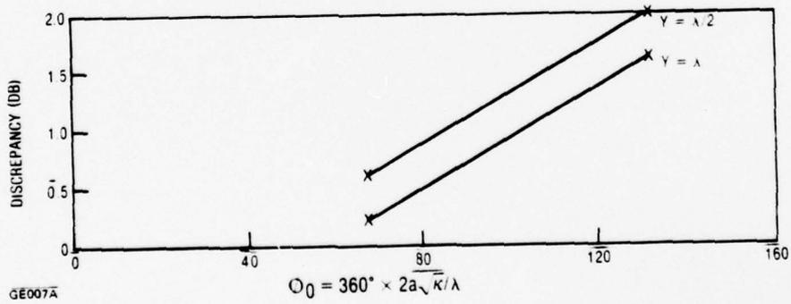
Figure 5-2. Maximum discrepancies for 10 in. wide slab from data in Figures 3-10 and 3-11.
