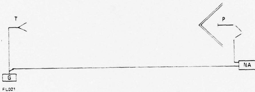
Figure 4-1. Apparatus for Transmittance Measurements. NA represents a network analyzer, G a generator, T a transmitting antenna, and P a probe antenna
