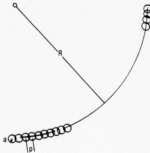
Figure 3-34. Approximating a Hollow Hemi-Cylinder with a Set of Solid Cylinders
