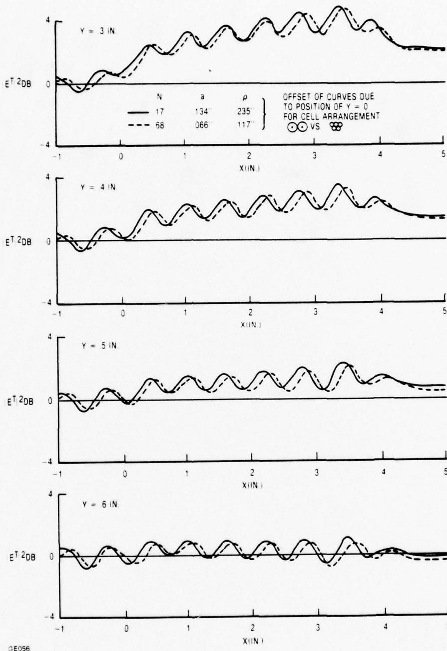
Figure 3-44. Computed Intensity Near Dielectric Slab for Grazing Incidence, Parallel Polarization
