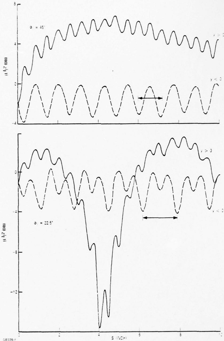
Figure 3-28a. Computed intensity of total field  $|E^T|^2$  inside hollow  $90^\circ$  wedge with  $1/8$  in. walls. Dielectric constant 2.6,  $N = 161$ ,  $\lambda = 1.259$  in. The arrows show spacings of nulls predicted by Equation 3-7. See Figure 3-7 for definition of  $\phi_1$ . (Sheet 1 of 2)
