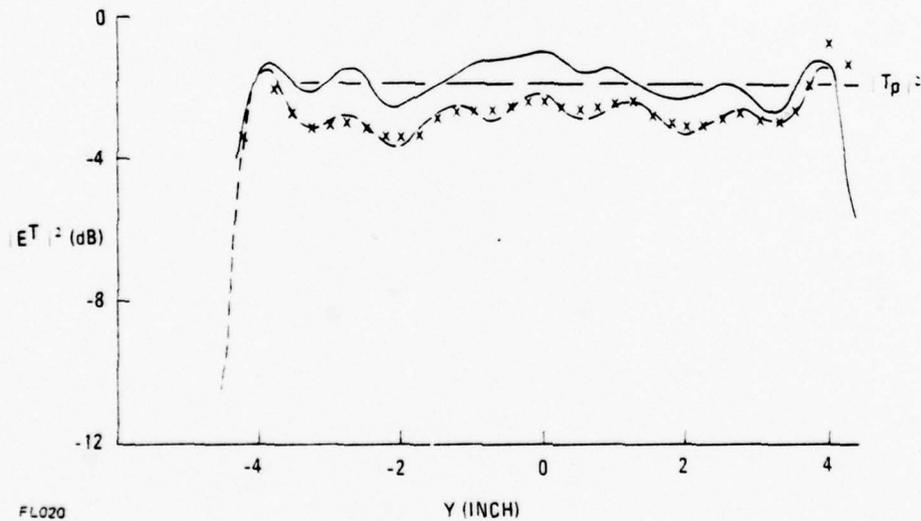
Figure 3-24. Intensity Behind Hollow Dielectric Wedge,  $\kappa = 2.6$ , With 18 in. x 18 in. Walls, Thicknesses 0.226 in. and 0.232 in. at  $\lambda = 1.259$  in. Measured with dipole probe (—). Calculated at  $x = 4.48$  in. (x), at  $x = 4.61$  in. ( $^\circ$ ).  $\rho = 0.25$  in.,  $a = 0.136$  in. for  $y < 0$ ,  $a = 0.130$  in. for  $y > 0$ .  $N = 81$ .
