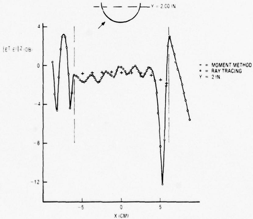
Figure 3-37. Power transmittance for the conditions of Figure 3-35, except with  $\phi_1 = 45^\circ$ . The dashed lines show the co-ordinates of the inner radome surface.
