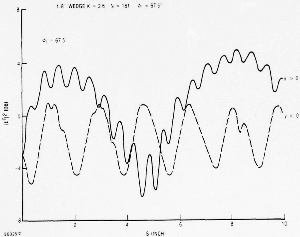
Figure 3-28b. Computed intensity of total field  $|E_T|^2$  inside hollow  $90^\circ$  wedge with  $1/8$  in. walls. Dielectric constant 2.6,  $N = 161$ ,  $\lambda = 1.259$  in. The arrows show spacings of nulls predicted by Equation 3-7. See Figure 3-7 for definition of  $\phi_i$ . (Sheet 2 of 2)
