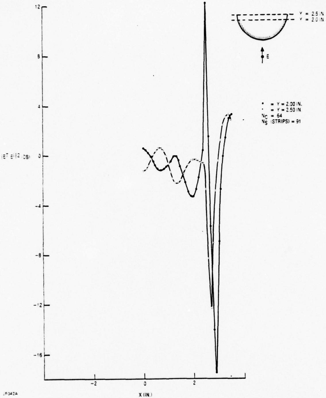
Figure 3-40. Power transmittance of hemi-cylinder with dielectric strips for  $\phi_i = 90^\circ$ . Inner diameter of hemi-cylinder 12.38 cm; thickness 0.32 cm; wavelength 3.2 cm. Computed by moment method. Radii of approximating cylinders were 0.180 and 0.086 cm. Data are symmetric about  $X = 0$ .
