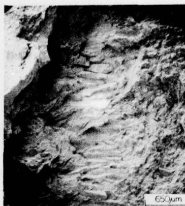
Fig. 6 — Columnar and adjacent refined grain areas showing predominantly transgranular fracture
