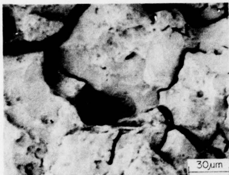
Fig. 5 — Intergranular fracture found in equiaxed grain area of weld bead 4
