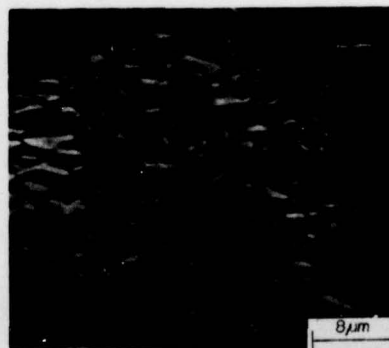
Fig. 17 — Backscattered electron display of the center of the inclusion seen in Fig. 16
