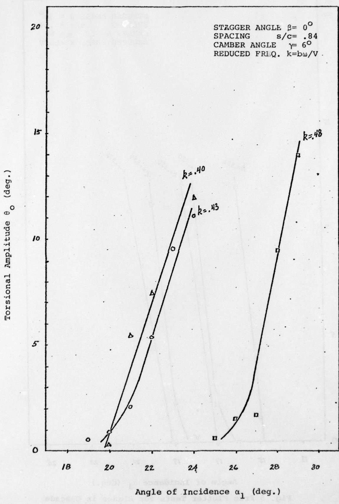
Fig. 4 Free Flutter Tests for Blades in Cascade
