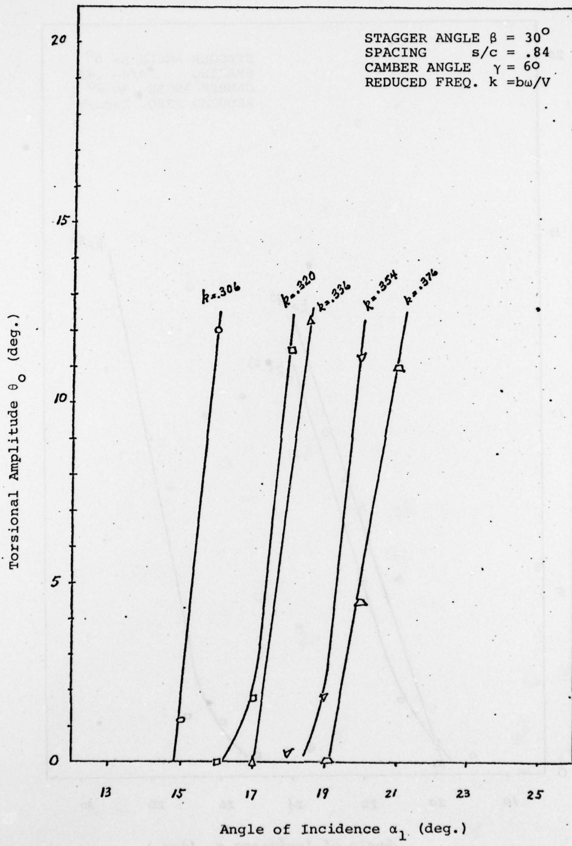
Fig. 5 Free Flutter Tests for Blades in Cascade
