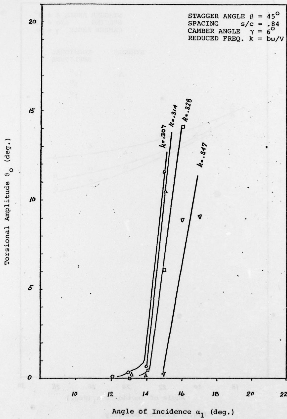
Fig. 6 Free Flutter Tests for Blades in Cascade
