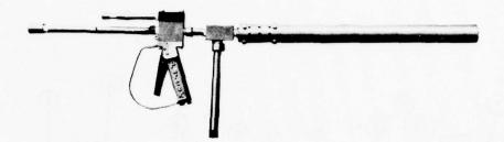
Designed specifically for underwater service, the Zero Thrust Gun utilizes an opposing jet to eliminate back thrust. The rear nozzle is mounted in a diffuser which dissipates the blast rendering it harmless.
