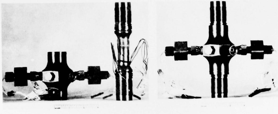
Figure 4. Biaxial external pressure sleeve and specimen.
