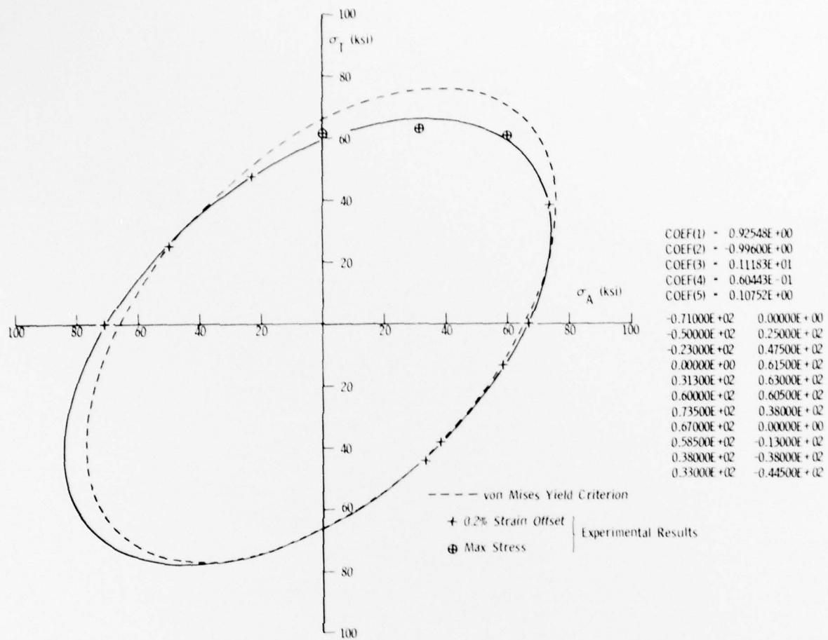
Figure 7. Yield surface for 2014-T651 aluminum alloy.
