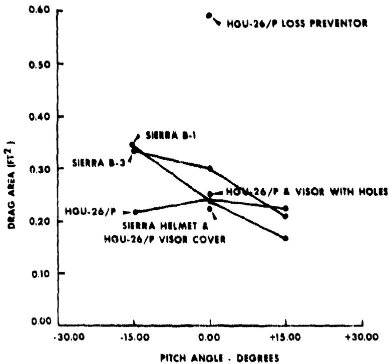
Figure 13. Drag vs. pitch.
