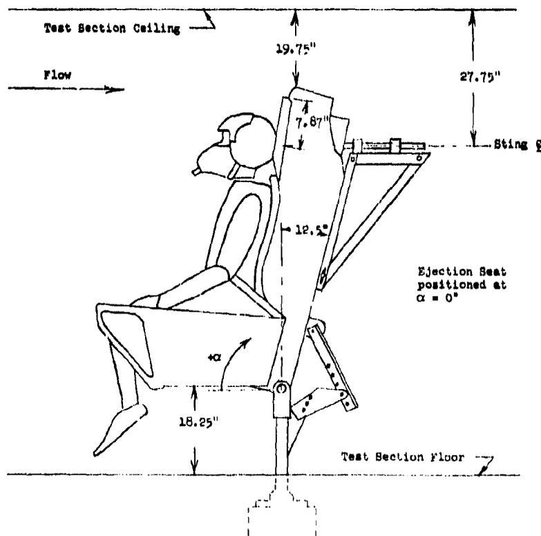
Figure 7. ACES-II ejection seat and dummy positioning.
