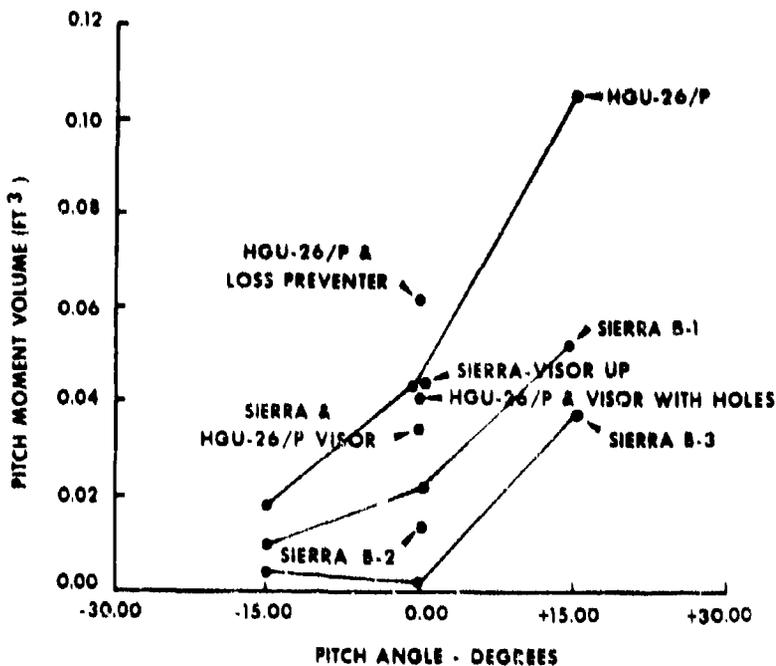
Figure 14. Pitch moment volume vs. pitch.
