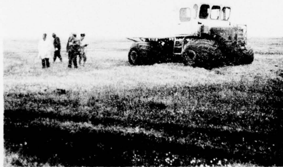
Figure B-1. Rolligon vehicle used for traffic tests. Ribbed (cleated) rubber tires; tire inflation pressure (and approximate ground contact pressure) between 0.2 and 0.3 kg/cm 2 (3 to 4 psi); no load, except for 2 men and fuel.
