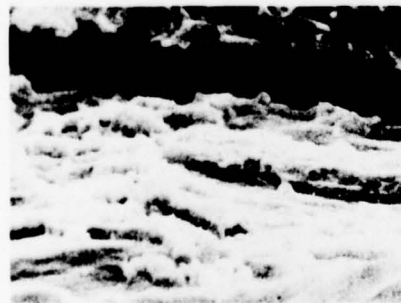
Figure 12.—SEM Photomicrograph—Anodize Time Variation—2024-T3 Clad
