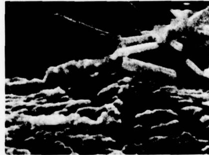
Figure 11.—SEM Photomicrograph—Anodize Time Variation—7075-T6 Bare
