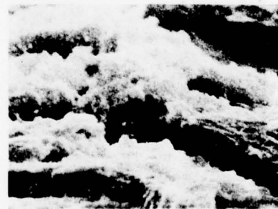
Figure 12.—SEM Photomicrograph—Anodize Time Variation—2024-T3 Clad
