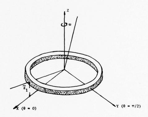
Figure 4. Motion of the Stator and the Definition of Rotating Coordinates
