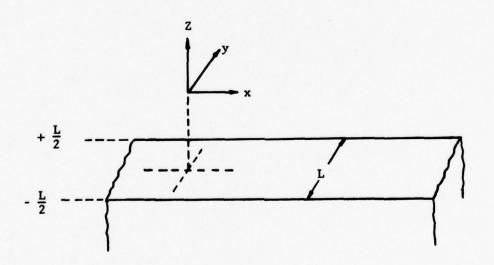
Figure 3. Axes of Coordinates for the Narrow-face Seal
