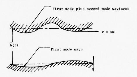
Figure 1. Sketch of Three Degree of Freedom Face Seal Model with Two Modes of Wayiness
