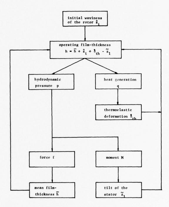
Figure 2. Block Diagram for Thermoelastic Analysis
