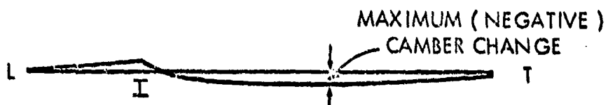
(b) MAXIMUM THINNING OCCURS CLOSE TO POINT OF INJECTION
