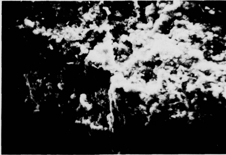
Figure 14. Specimen INN-13-PC - Low Cycle Fatigue, PC Loading Test Temperature - 1700°F Air Material - IN-100, Total Strain Range - 0.0058, 139 Cycles Test Time - 87.3 Hrs., 1000X A Compression Dominated Hold can Damage The Grain Boundary Fatigue Indications, Particularly in an Air Environment.
