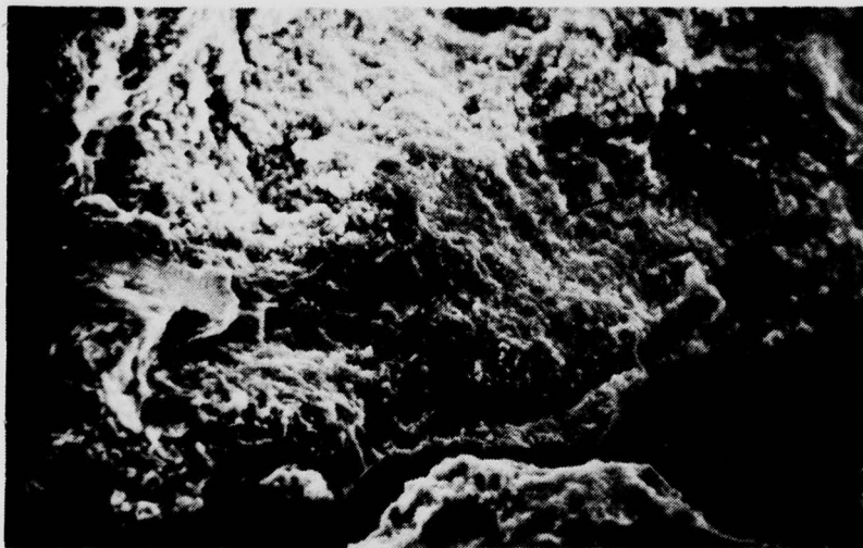
Figure 15. Specimen INN-9-CP - Low Cycle Fatigue, CP Loading Test Temperature - 1700°F Air Material - IN-100, Total Strain Range - 0.0041, 1100 Cycles Test Time - 159.3 Hrs., 400 X Reverse Loading Can Damage the Dimples Found in Grain Boundary Fatigue, But is Less Damaging in a Tension Hold Dominated Fatigue Load.
