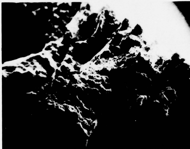
Figure 9. Specimen INN-3-PP - Low Cycle Fatigue, PP Loading Test Temperature - 1700° Air Material - IN-100 Total Strain Range - 0.0092, 96 Cycles Top 400X, Bottom 50X Dominant Transgranular (Interdendritic) Fatigue Note Some Slip Planes (Arrow).
