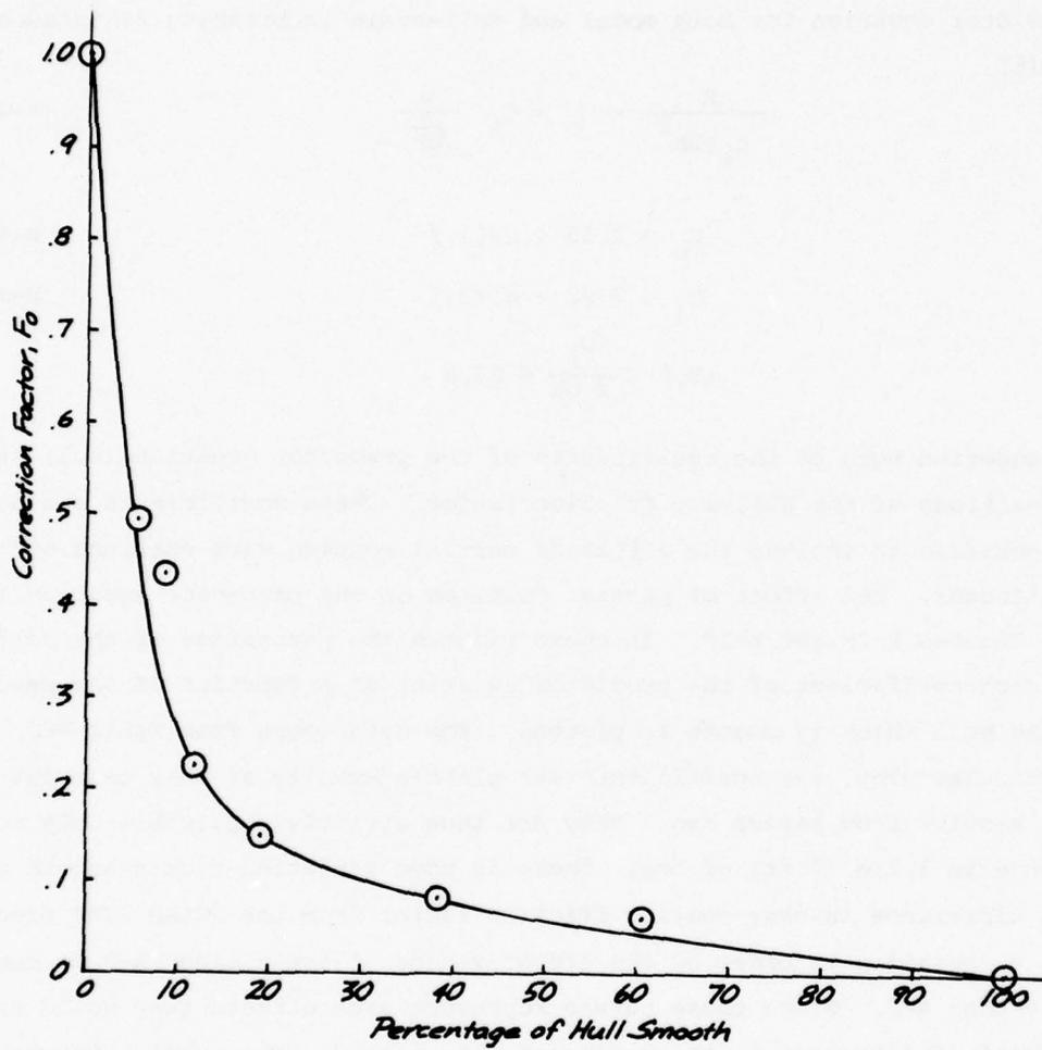
Figure B-18 Effect of Coating on Predictor Intercept
