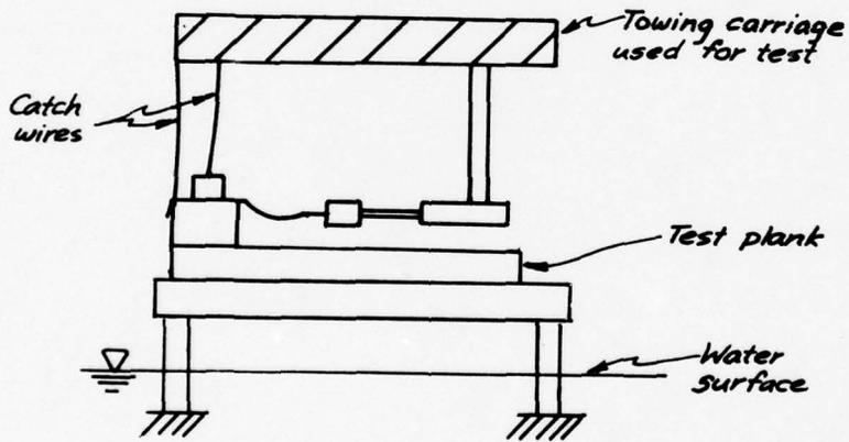
Figure B-3 Set-up for Friction Tests Inside Model Basin
