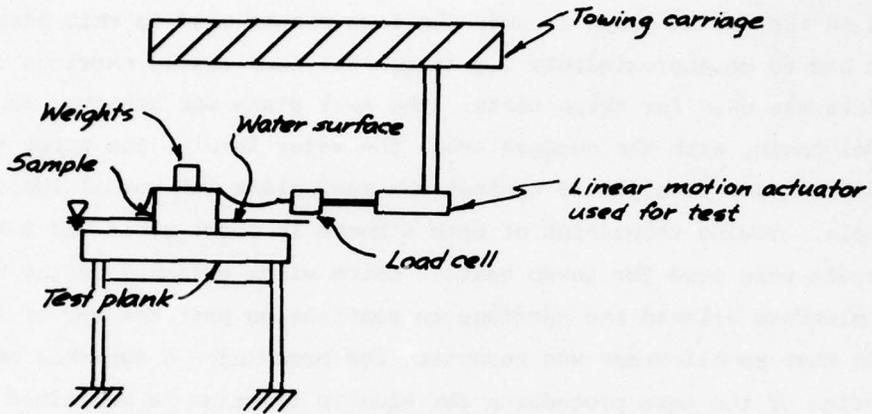
High Speed Friction Test
