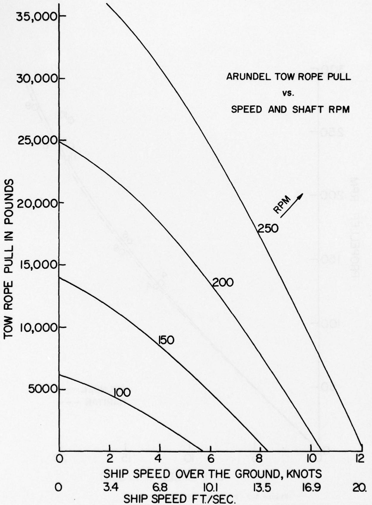
Figure A-4 ARUNDEL Tow Rope Pull Performance Curves
