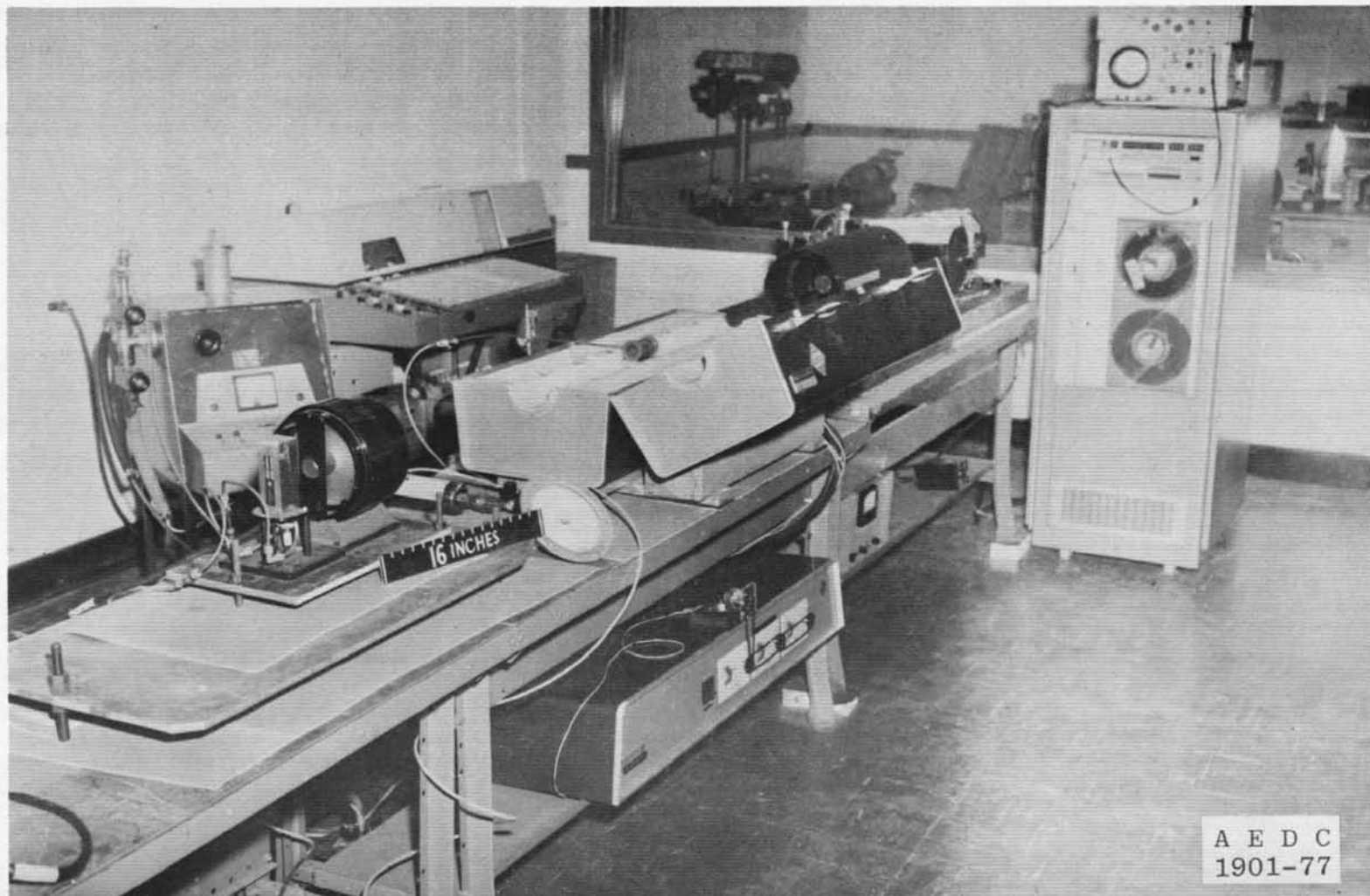
Figure 1. Interferometer spectrometer and data acquisition system.
