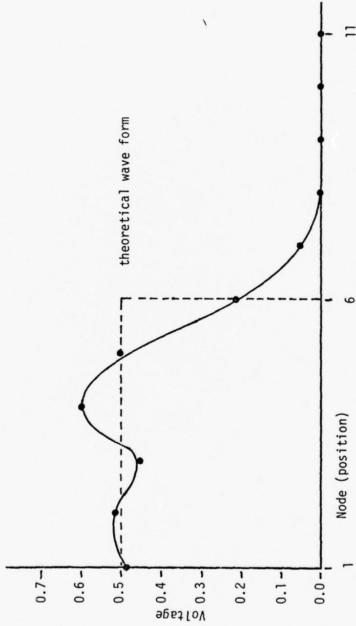
Figure 2-17. Voltage versus position for a 10 section line,  $\Delta t = .01$ ,  $t = 0.5$
