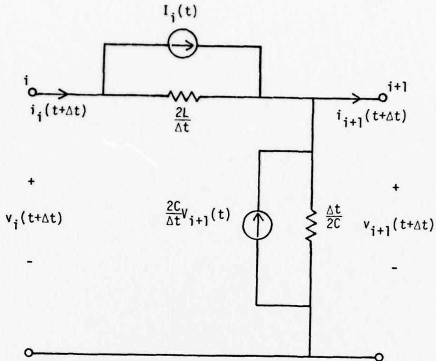
Figure 2-3. Typical transmission line equivalent section with all current sources
