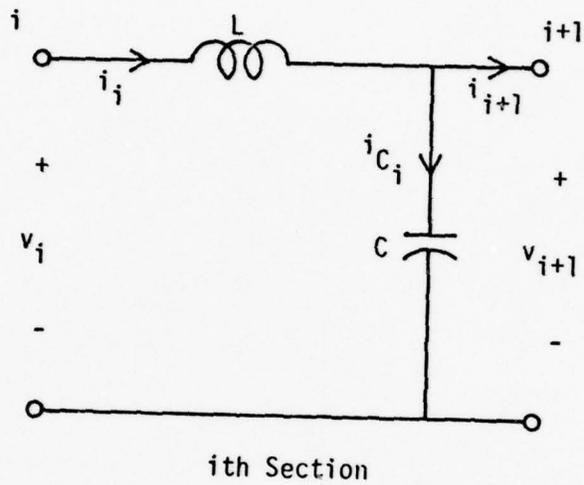
Figure 2-1. Typical lossless transmission line section
