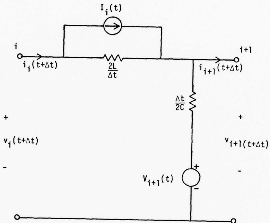
Figure 2-2. Typical lossless transmission line equivalent section
