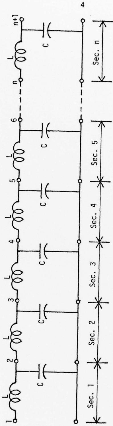
Figure 1-1. Transmission line represented by  $n$ -sections and  $n+1$  nodes
