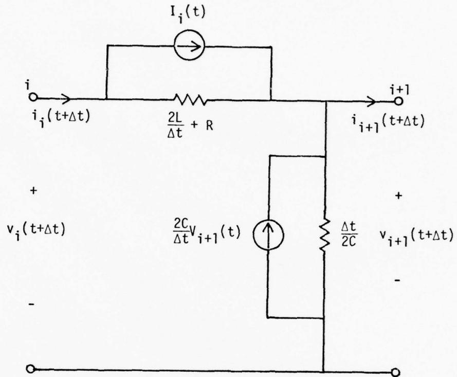
Figure 2-23. Typical lossy transmission line equivalent section
