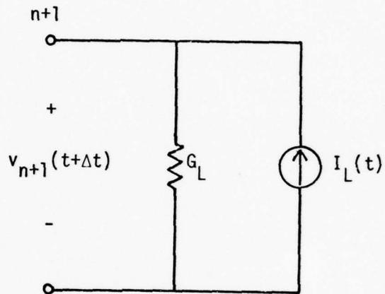
Figure 2-8. Equivalent receiving-end model
