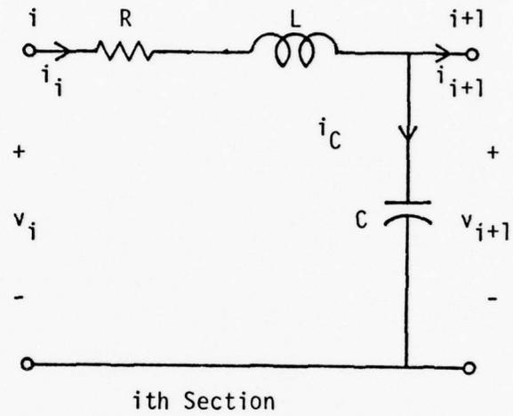
Figure 2-22. Typical lossy transmission line section
