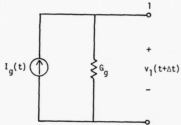
Figure 2-7. Combined equivalent source model
