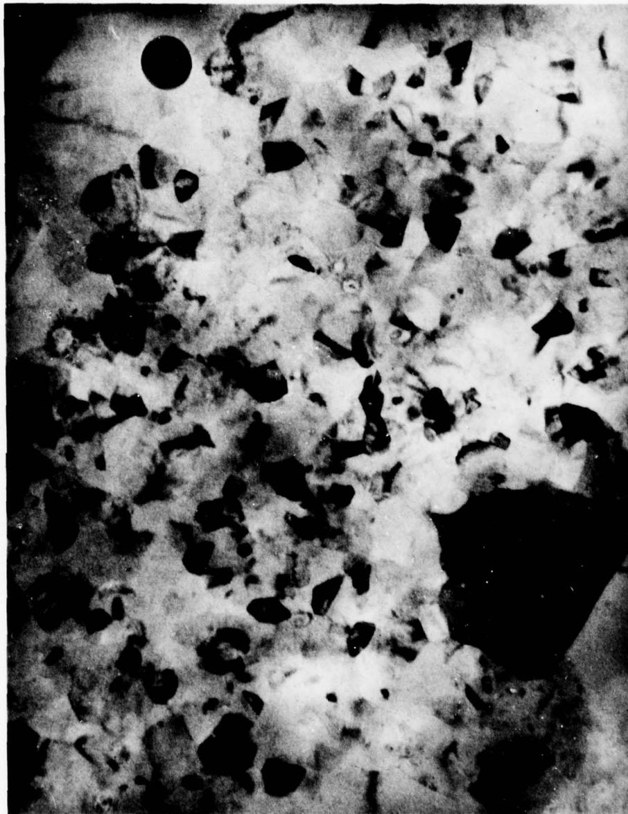
Figure 11 TEM micrographs of the splat cooled specimen of Al-4.5% Cu alloy shown in Figure 10. Magnification: 75,000X.
