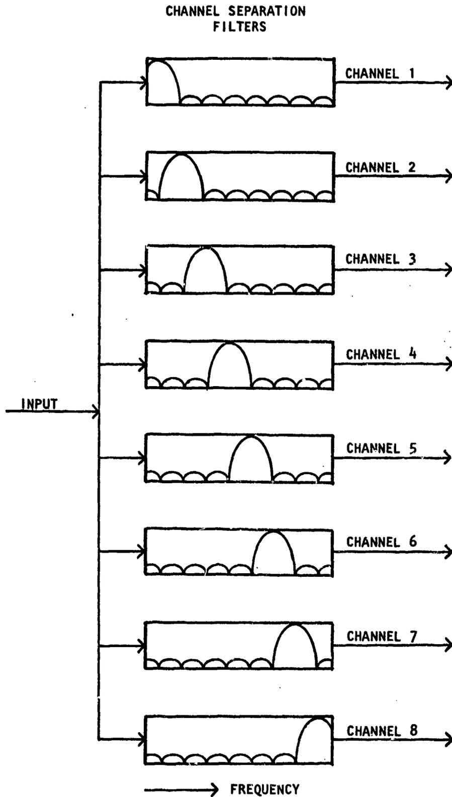
FIGURE 3-17. CHANNEL SEPARATION FOR 8 CHANNEL TAYLOR PROCESSING
