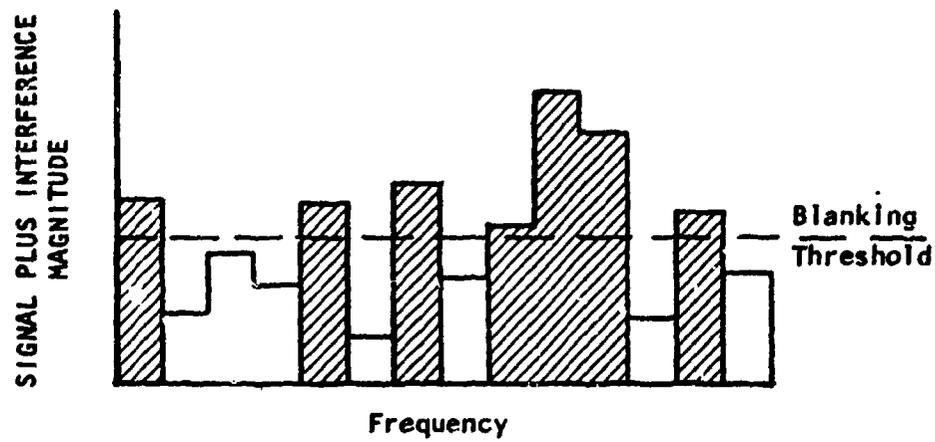
FIGURE 3-13. OPERATION OF NON-COHERENT FREQUENCY BLANKER IN NARROW BAND AND WIDE BAND INTERFERENCE
