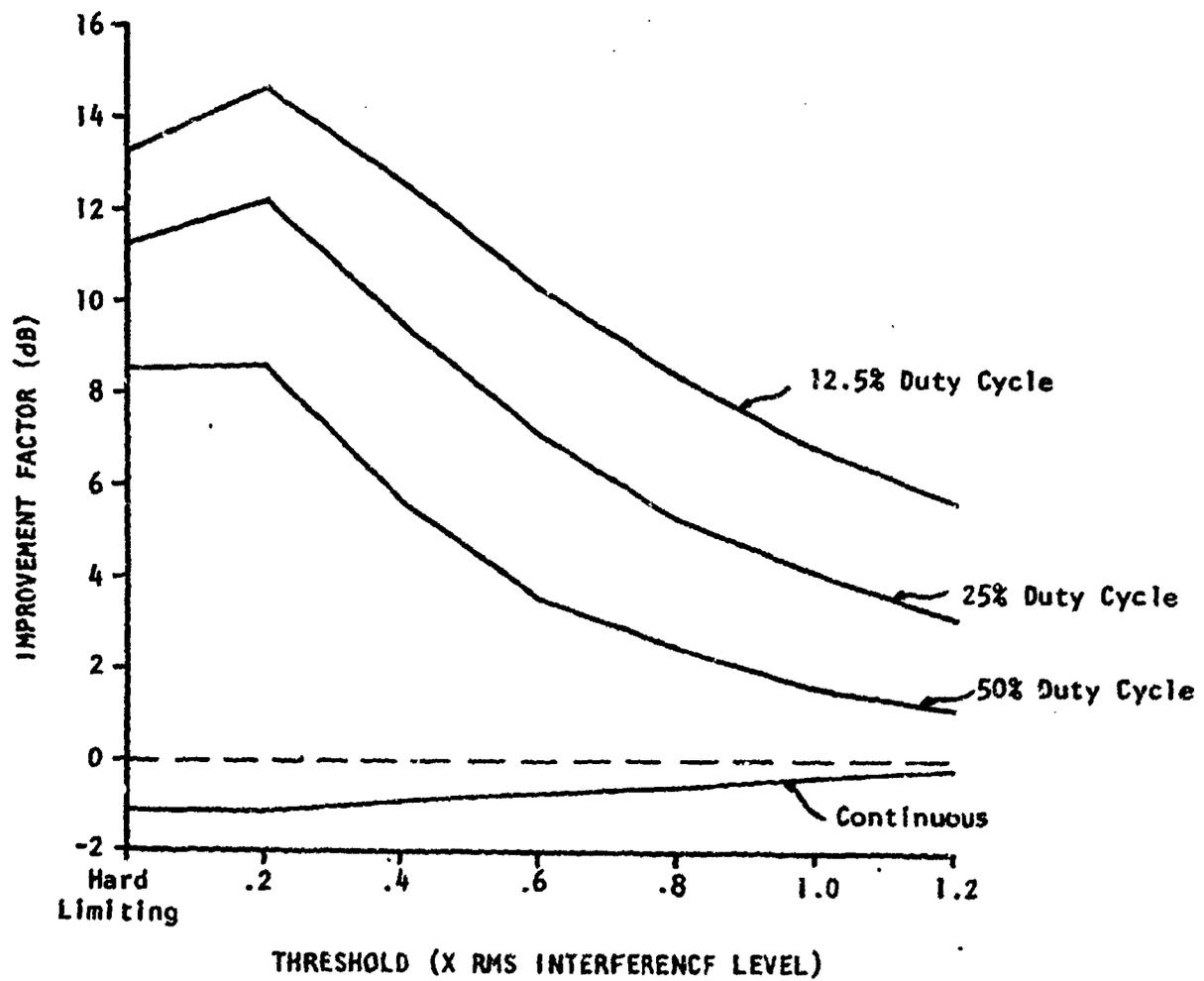
FIGURE 3-14. NON-COHERENT CLIPPING IMPROVEMENT FACTOR FOR WIDE BAND PULSED GAUSSIAN JAMMING, 0 dB S/N, 18 dB J/N
