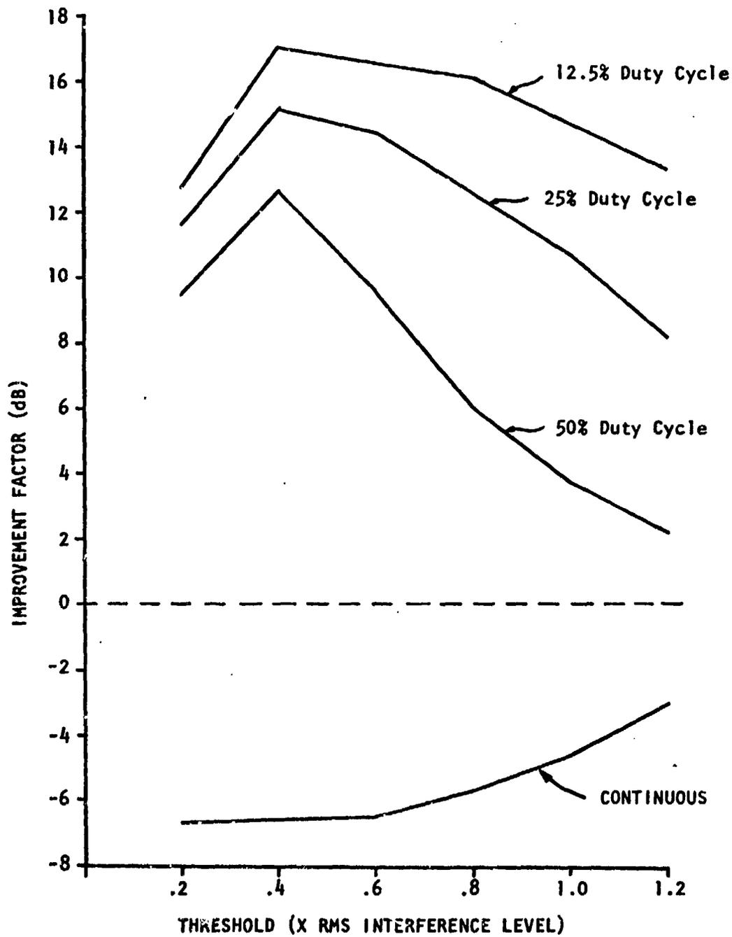
FIGURE 3-15. NON-COHERENT BLANKING IMPROVEMENT FACTOR FOR WIDE BAND PULSED GAUSSIAN JAMMING, 0dB S/N, 18 dB J/N
