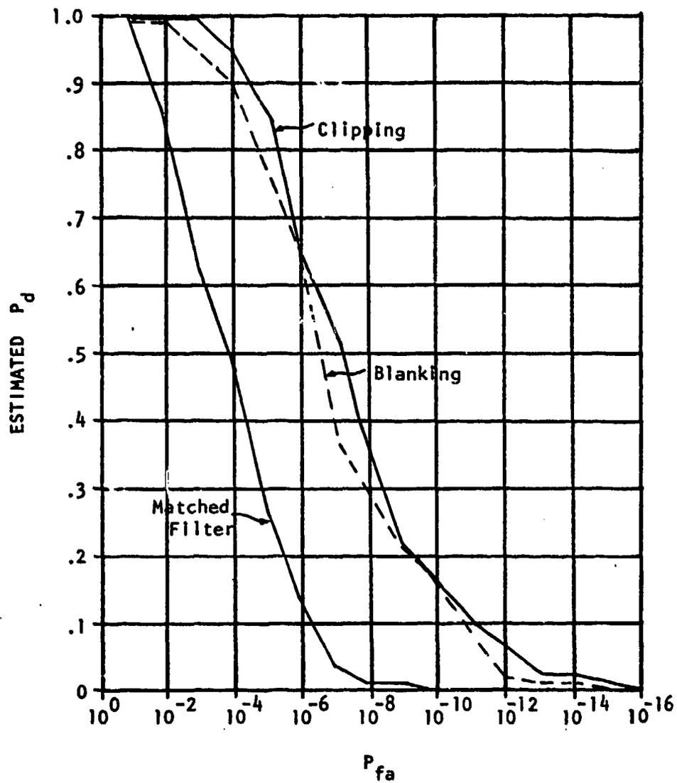
FIGURE 3-11. DETECTION PERFORMANCE FOR NON-COHERENT CLIPPING/BLANKING FOR 0 dB S/N, 15 dB J/N, AND 10% JAMMER BANDWIDTH
