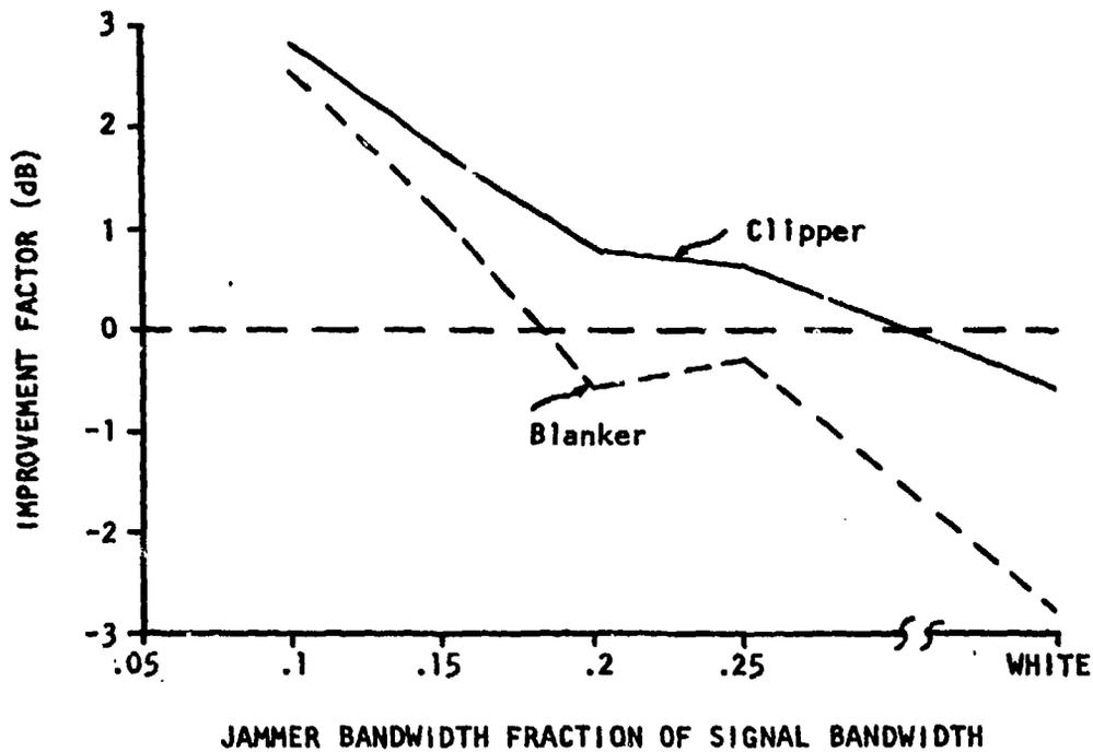
FIGURE 3-12. NON-COHERENT CLIPPER/BLANKER PERFORMANCE AS A FUNCTION OF JAMMER BANDWIDTH, 0 dB S/N and 15 dB J/N
