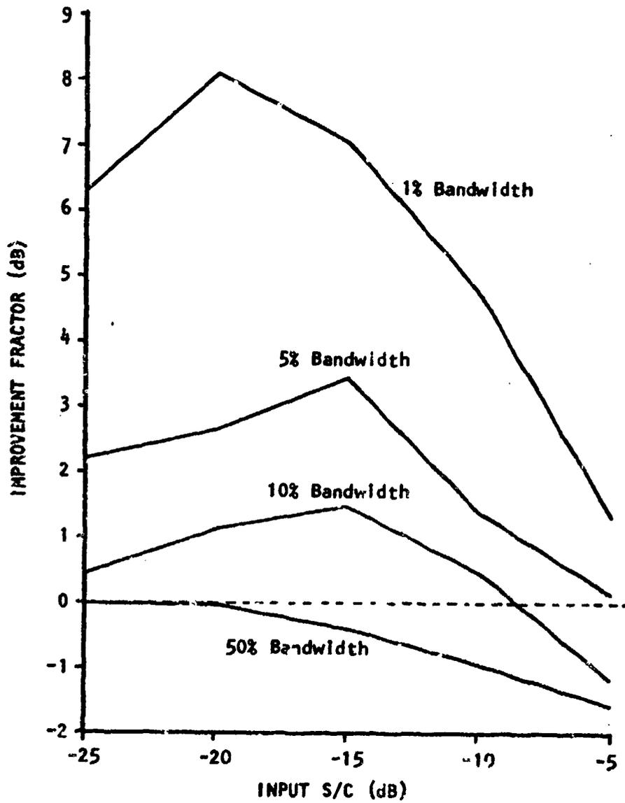
FIGURE 3-21. PEAK-NORMALIZING AGC PROCESSOR PERFORMANCE AS A FUNCTION OF JAMMER BANDWIDTH
