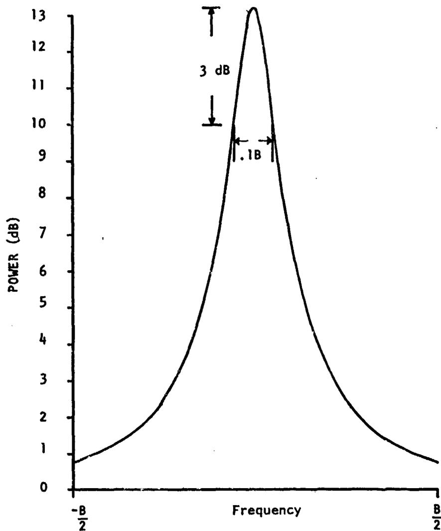
FIGURE 3-2. INTERFERENCE POWER SPECTRUM FOR 10 dB JAMMER-TO-NOISE RATIO, 10% JAMMER to SIGNAL BANDWIDTH.
