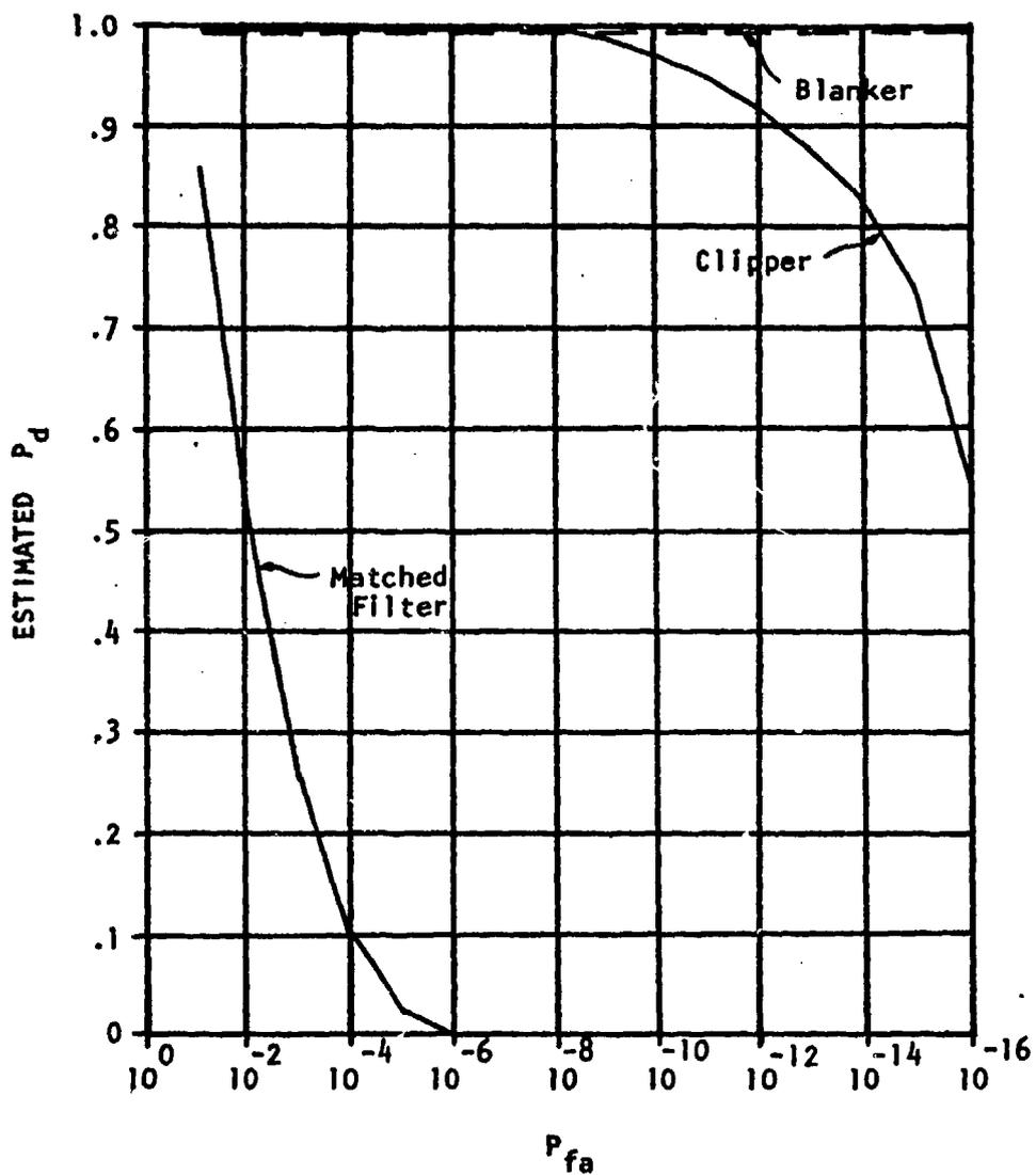
FIGURE 3-16. DETECTION PERFORMANCE FOR NON-COHERENT CLIPPING/BLANKING IN 50% DUTY CYCLE WIDE BAND JAMMING, 0 dB S/N, 18 dB J/N
