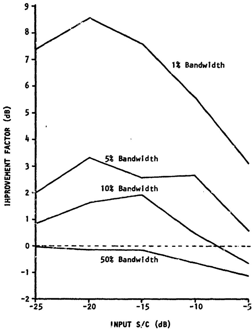
FIGURE 3-22. RMS-NORMALIZING AGC PROCESSOR PERFORMANCE AS A FUNCTION OF JAMMER BANDWIDTH
