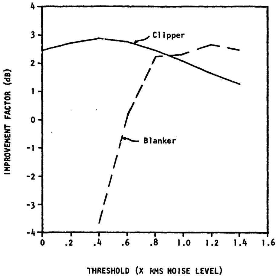
FIGURE 3-9. IMPROVEMENT FACTORS FOR THE NON-COHERENT CLIPPER/BLANKER FOR 0 dB S/N, 18 dB J/N, AND 10% JAMMER BANDWIDTH
