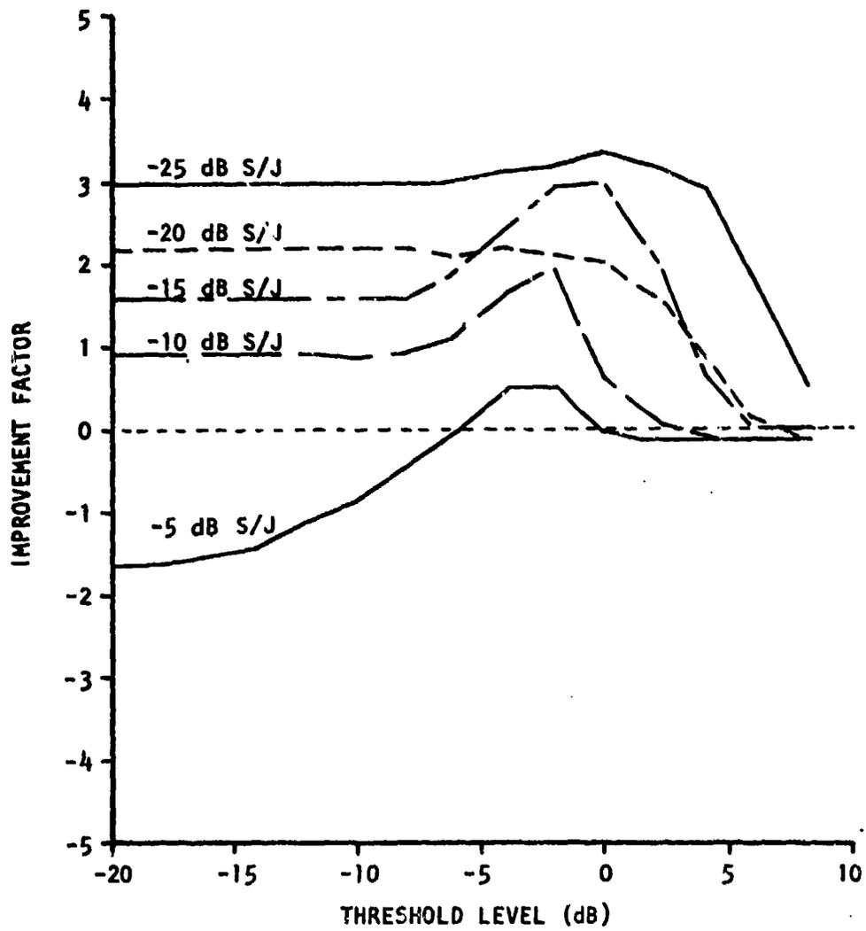
FIGURE 3-19. THRESHOLD SENSITIVITY FOR TAYLOR PROCESSING, 5% JAMMER BANDWIDTH
