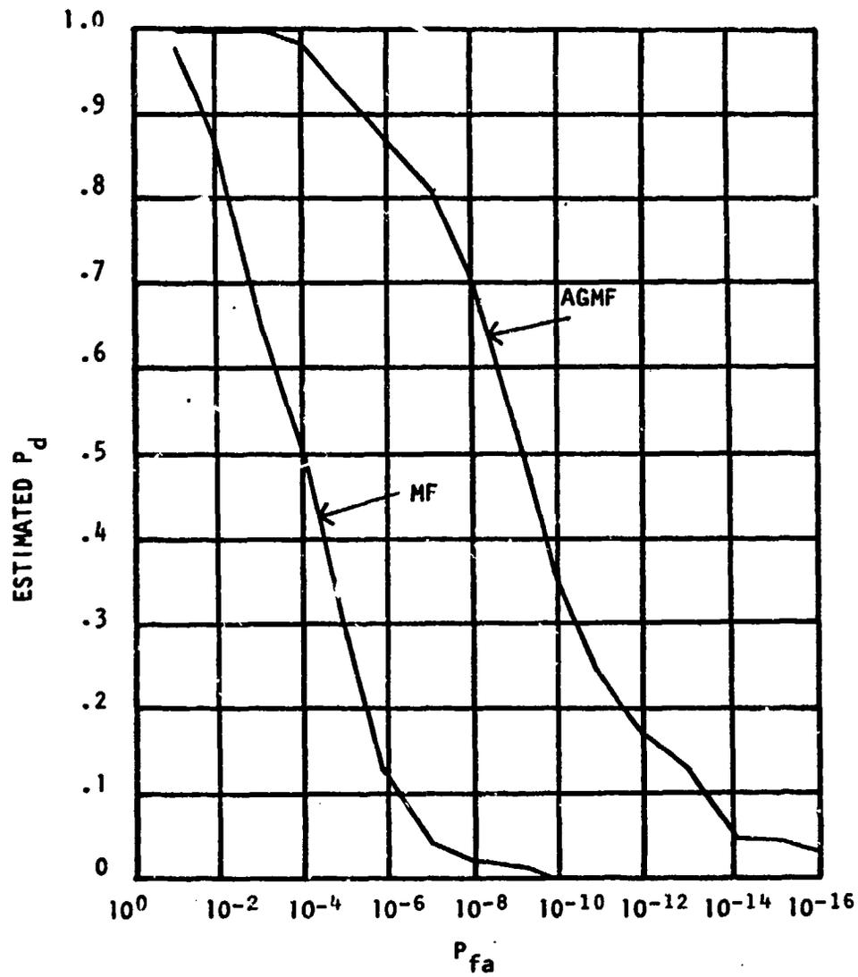
FIGURE 3-5. DETECTION PERFORMANCE OF AGMF FOR 10 DB S/N, 25 dB J/N, AND 10% JAMMER BANDWIDTH
