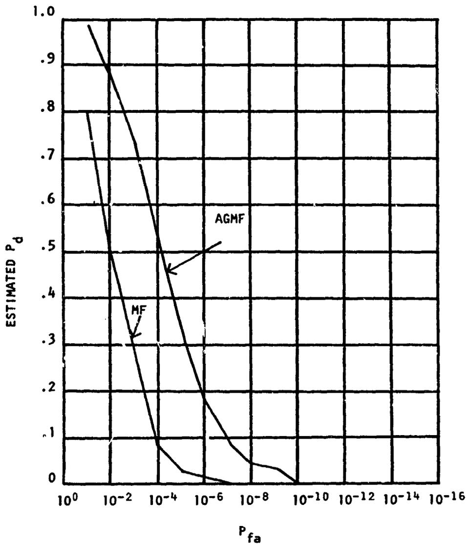
FIGURE 3-6. DETECTION PERFORMANCE OF AGMF for 0 dB S/N, 18 dB J/N, and 10% JAMMER BANDWIDTH
