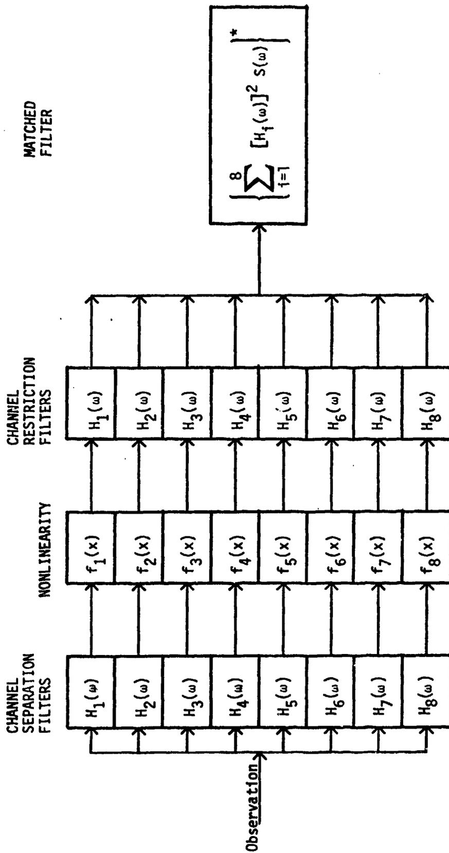
FIGURE 3-18. DIAGRAM OF TAYLOR PROCESSING SIMULATION
