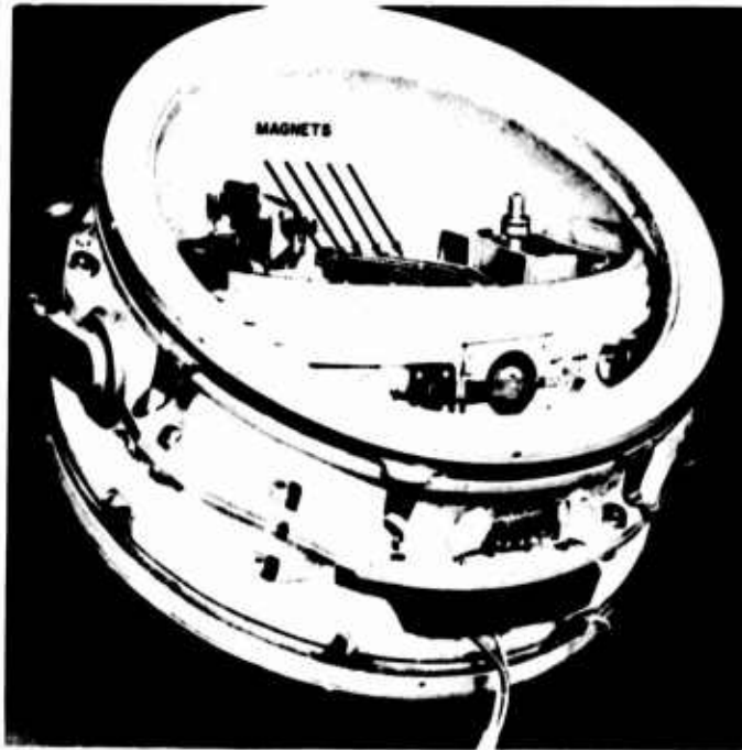
Figure 44.—Early German magnetic mine firing device.
