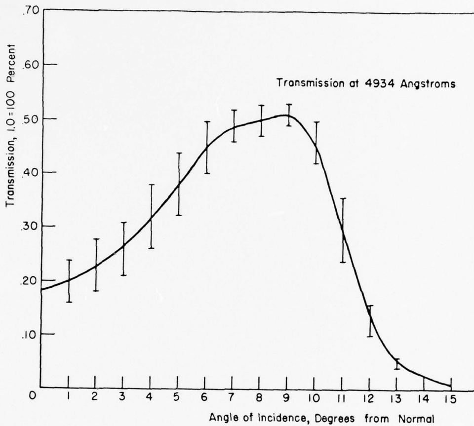
Figure 4.3 Variation of transmission with angle of incidence for DNA 4934A filter.
