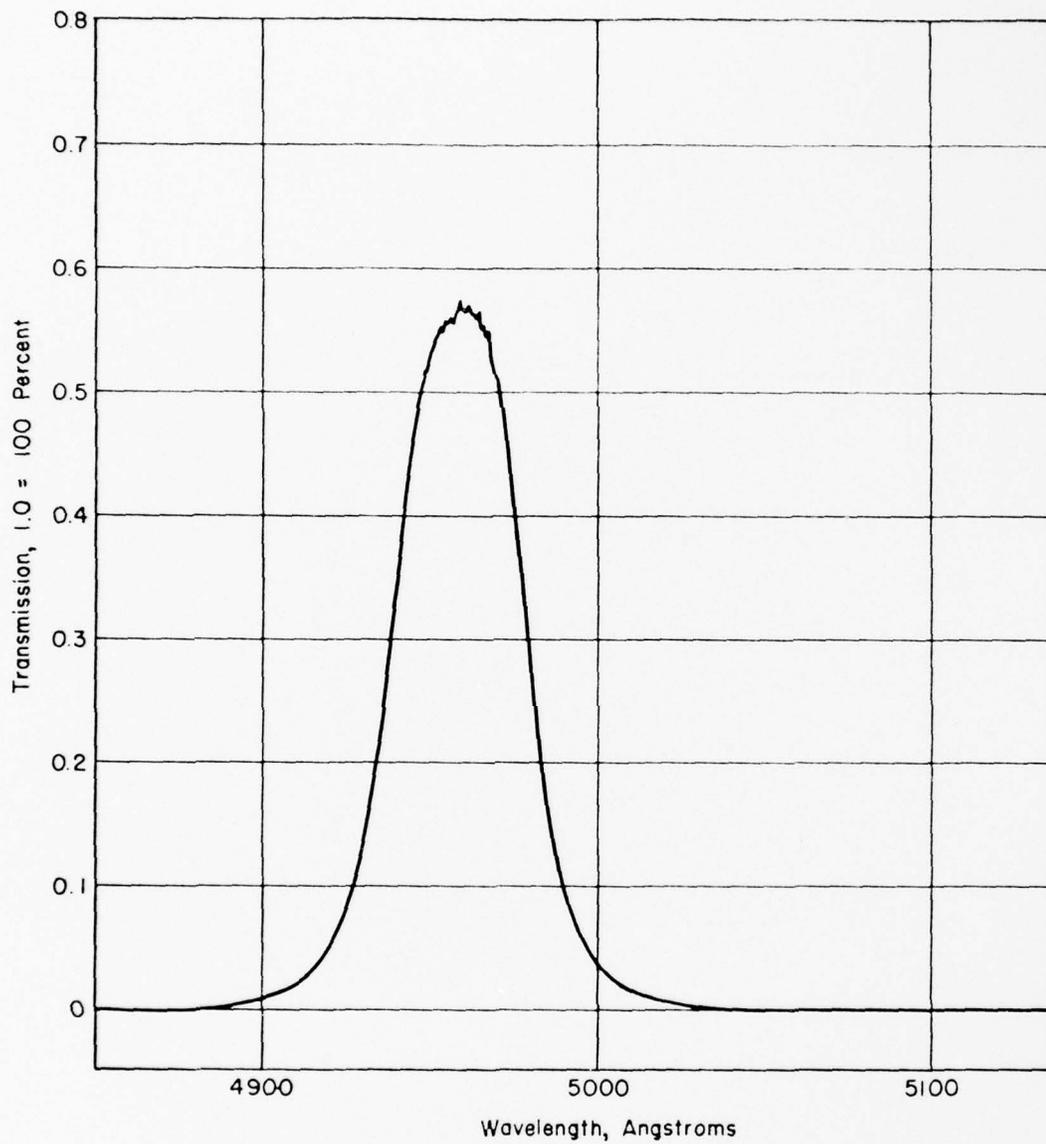
Figure 4.2 Transmission of DNA 6" diameter 4934A interference filter centered at 4960A at zero incidence angle.
