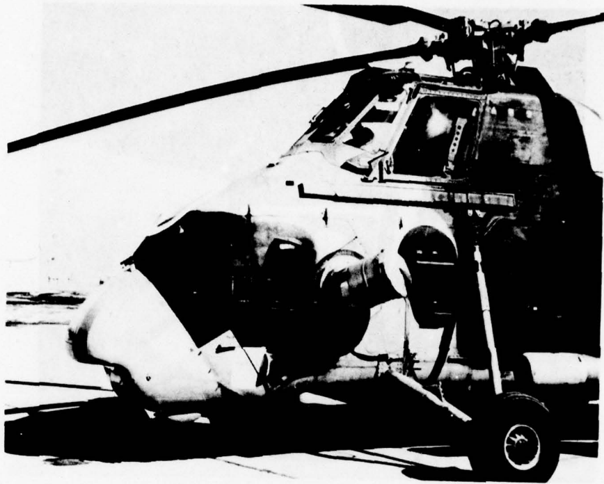
Slide 5. Downward-facing Plenum Intake.
