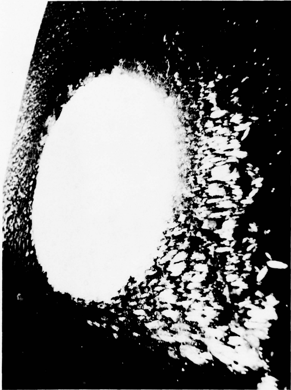
ICE ACCUMULATION ON THE ENVIRONMENTAL CONTROL UNIT SCREEN AFTER 60 MINUTES IN THE SPRAY RIG AT -4.0^{\circ}\text{C}
