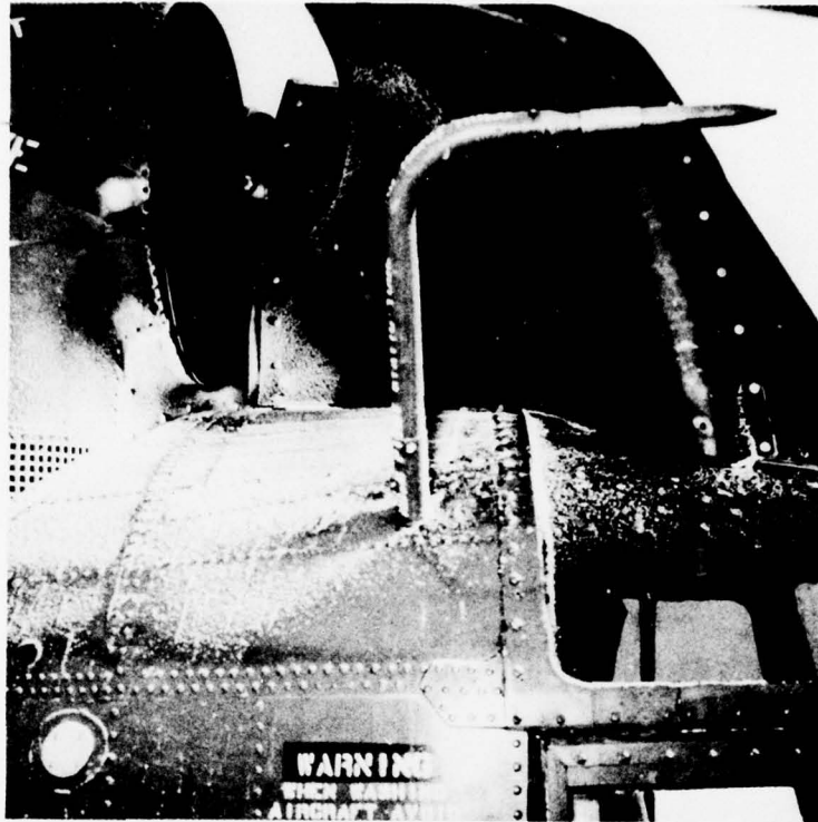
Figure 10 Frost Build-up on H-3 Shield With Aerofairing Installed
