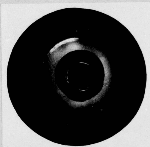
Figure 41. Back Reflection X-ray Pattern - Sample of Figure 39 after quenching from 920°C.
