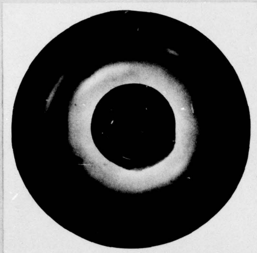
Figure 39. Back Reflection X-ray Pattern - 20% cold Rolled 3 Al-5 Cr- Ti Alloy Sheet
