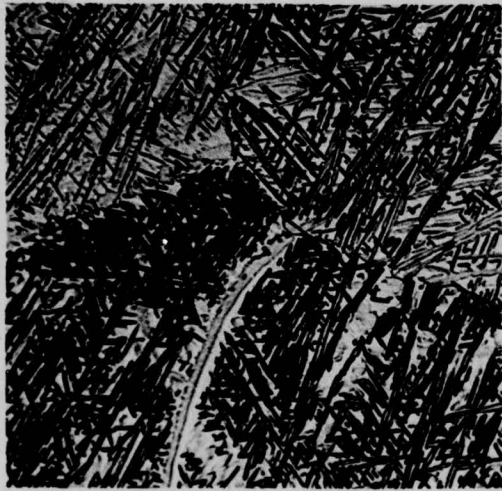
Fig. 18 Reheated to 850° Quenched 500X
