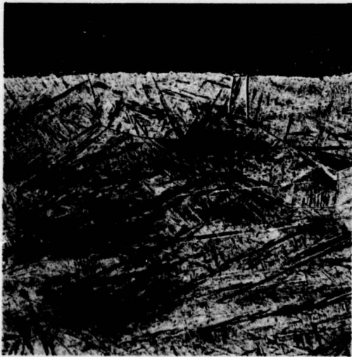
Fig. 6 \frac{1}{2} hr 1000°C Quenched 50X
