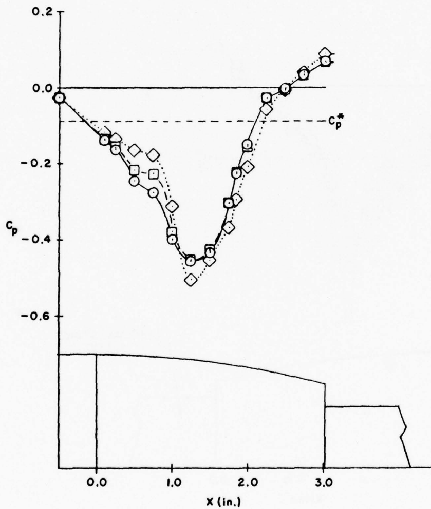
Figure 39. Mass Injection Effect on Boattail and Base Pressure Coefficients for NPR=2, D_S > 1"
