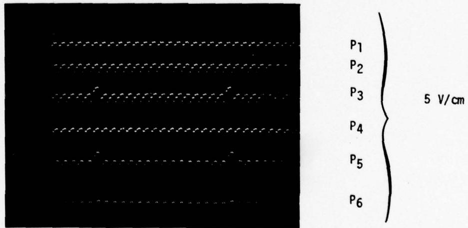
Figure 5-19. Input to the 2-Word, 3 Bit Multiplier
