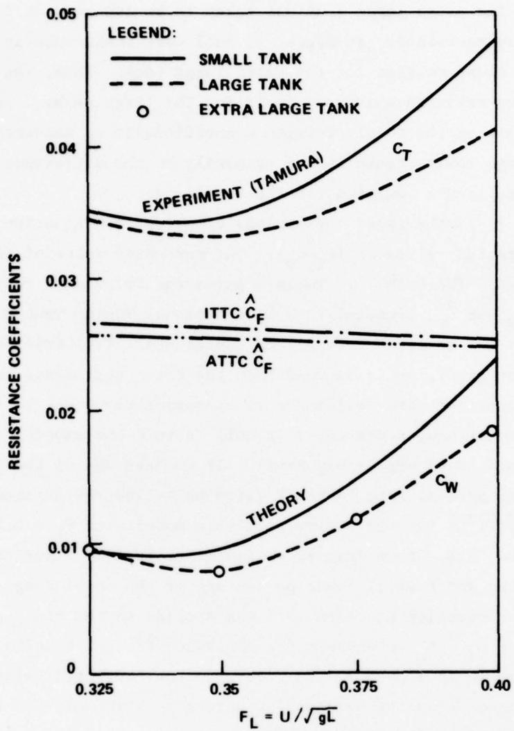
Figure 1 - Resistance Coefficients,  $C_T$ ,  $C_W$ , and  $\hat{C}_F$
