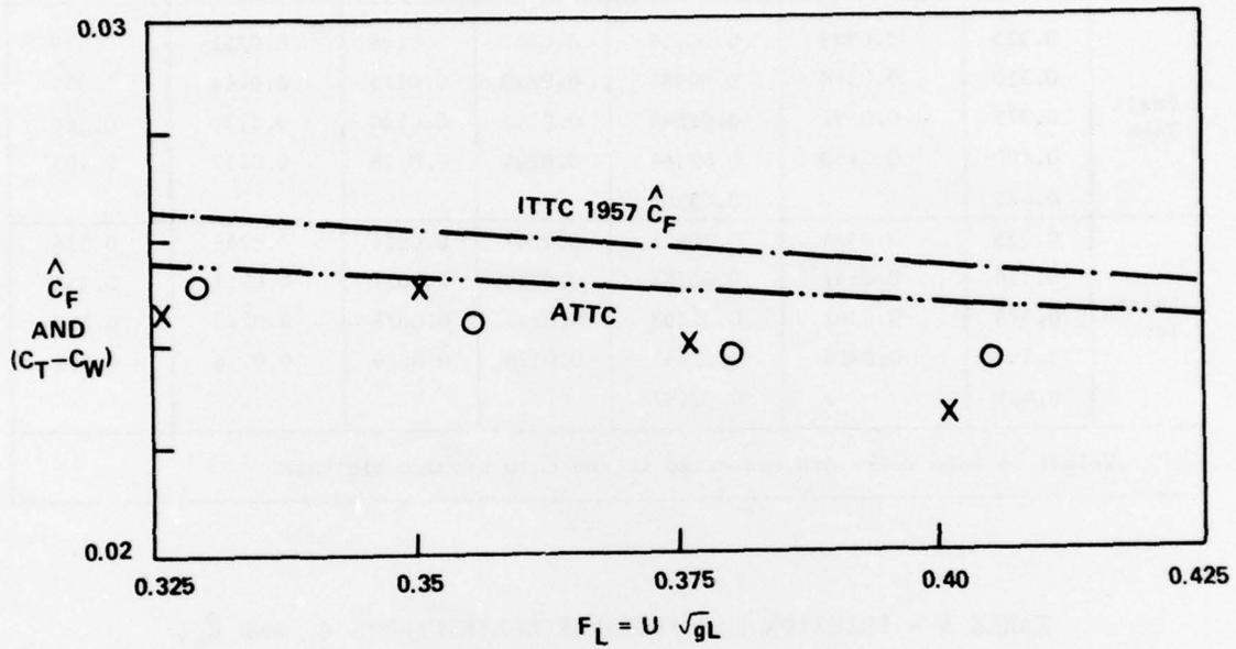
Figure 2 - Corrected Values of  $(C_T - C_W)$  from Small Tank
