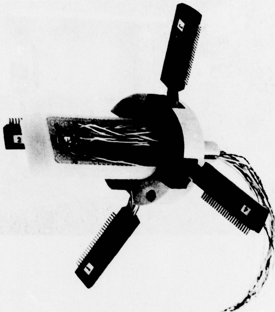
Figure A-17. Rotating Thermocouple Multiplexer.
