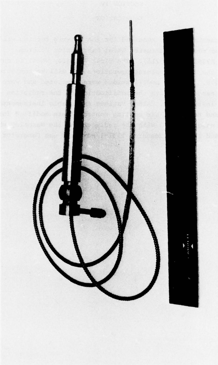
Figure 15. Pyrometer Manufactured by Vanzetti Corporation.
