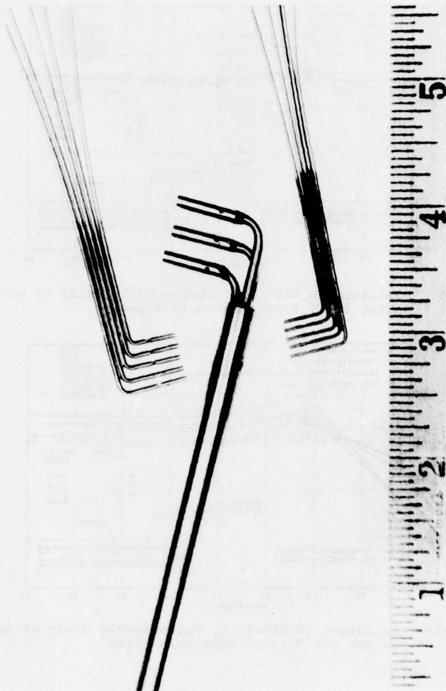
Right to Left 0.045-In.-OD Rake, 0.125-In.-OD Rake, 0.032-In.-OD Rake.
