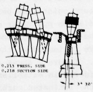
Figure 1. Test Section Schematic for TFE731-3.
