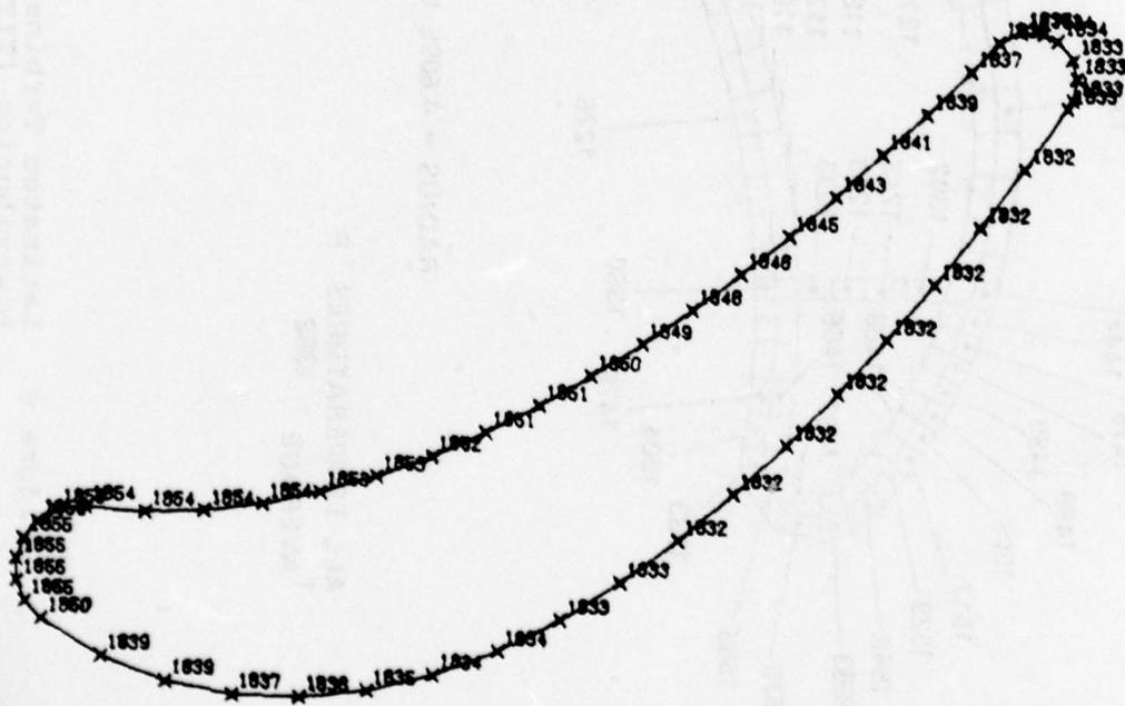
Figure 7. Laminated Turbine Blade Adiabatic Wall Temperatures at 2000°F T.I.T.
