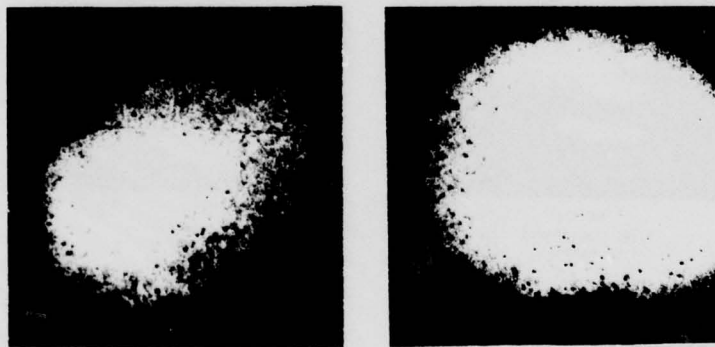
Fig. 18. Images independently reconstructed from a double reference beam hologram recorded in the Fig. 17 apparatus with laser pulses separated by 10 microseconds. MX-70 propellant at 34 atmospheres.
