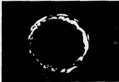
Figure 32. Far field radiation pattern observed from (a) short piece of fiber without a connector, (b) short piece of fiber with a good connector, (c) short piece of fiber with a poor connector. In all cases, the high-order modes of the fiber are excited at the input.
