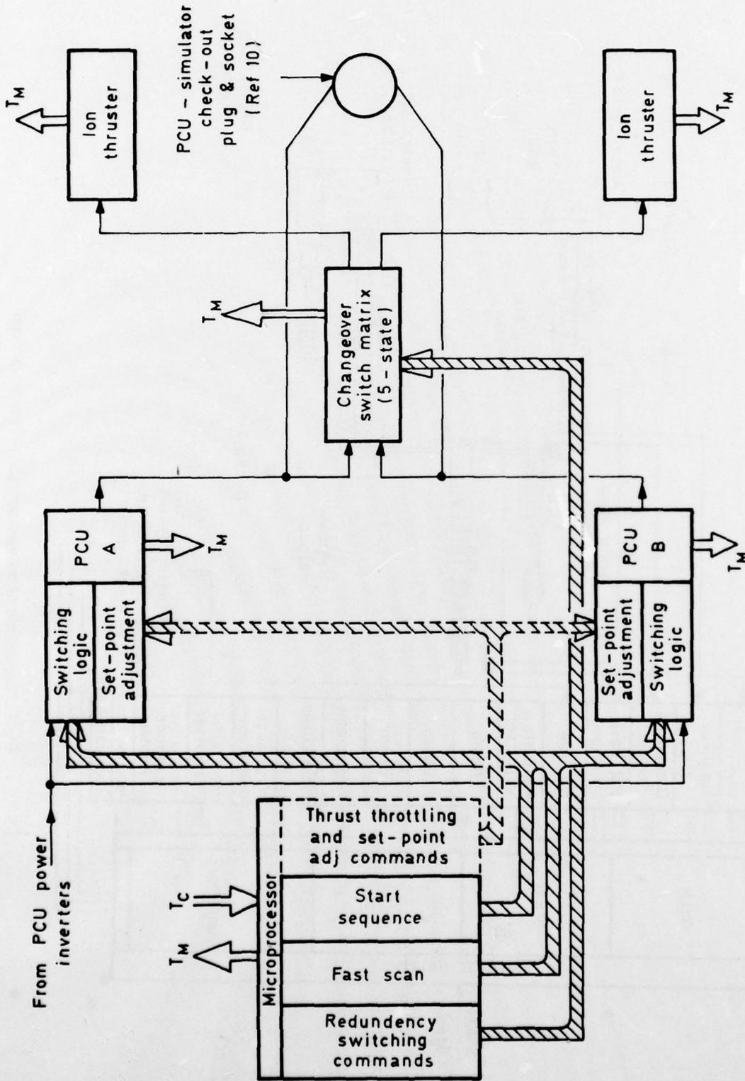
Fig 2 Ion thruster/PCU switching and control schematic
