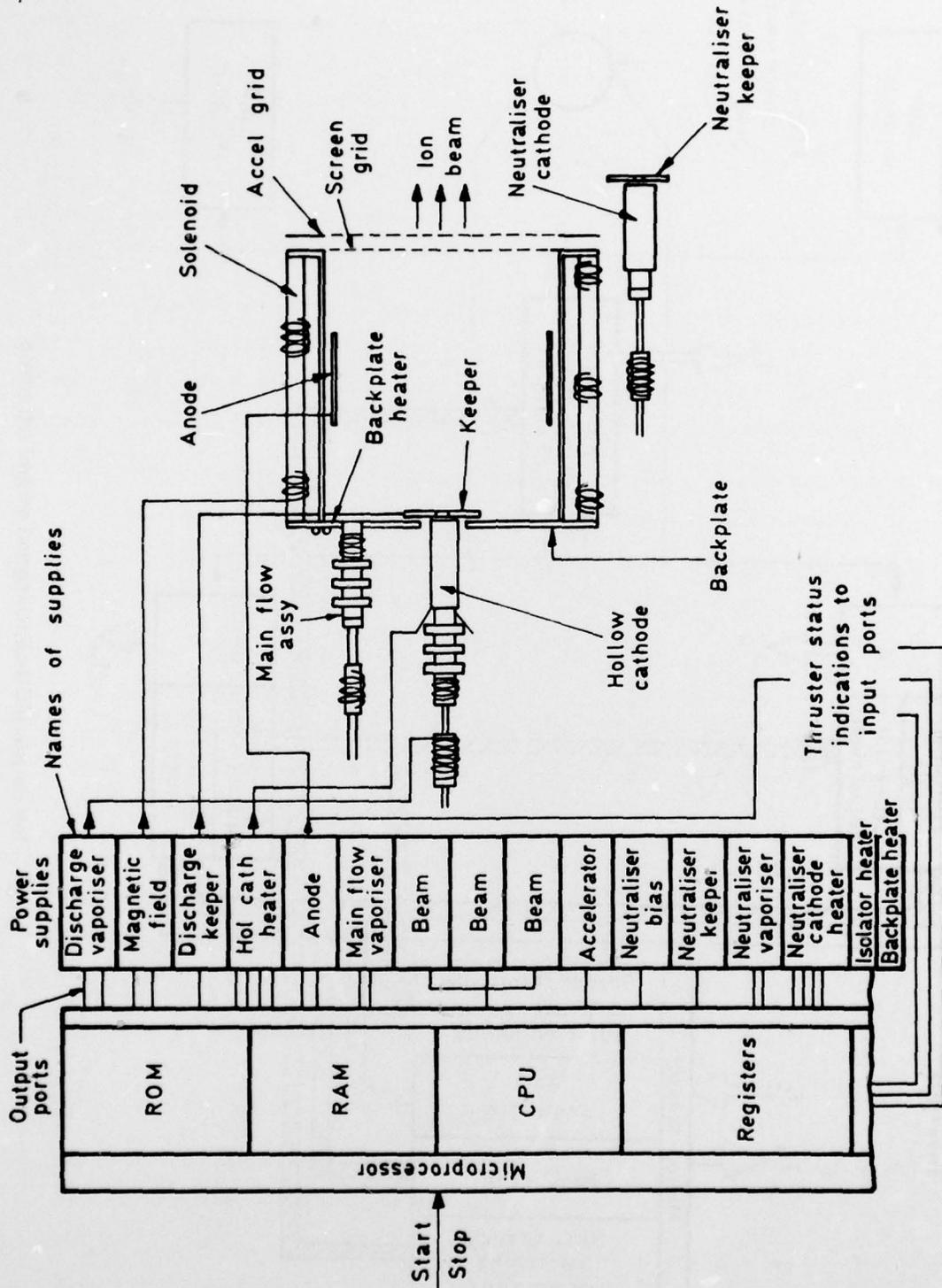
Fig 1 Schematic of microprocessor — PCU — thruster
