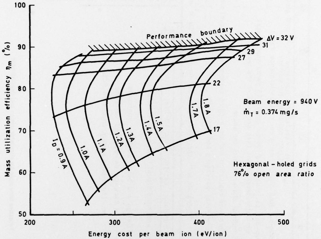
Fig 9 Performance map of T4A thruster, showing performance boundary
