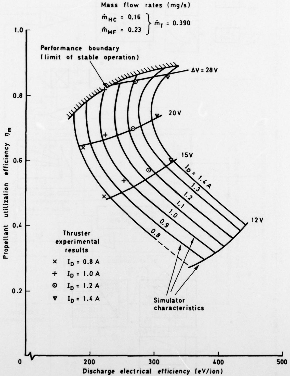
Fig 4 Comparison of simulator performance with thruster data
