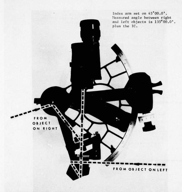
FIGURE 5. SURVEY SEXTANT WITH PENTA PRISM IN NORMAL-USE POSITION. The light beams show how the penta prism adds  $90^{\circ}$  to the index arm reading when the penta prism is inserted with a clockwise turn.
