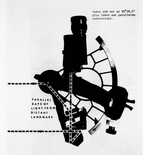
FIGURE 6. SURVEY SEXTANT WITH PENTA PRISM IN ADJUST POSITION. The light beams show how the pentaprism subtracts  $90^{\circ}\,00.0$ ' from the index arm reading when the pentaprism is inserted with a counterclockwise turn.
