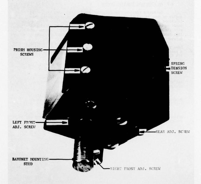
FIGURE 12. OBLIQUE VIEW OF PENTA PRISM SHOWING ADJUSTMENT SCREWS
