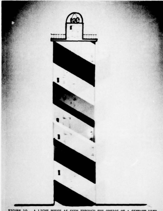
FIGURE 10. A LIGHT HOUSE AS SEEN THROUGH THE OPTICS OF A SEXTANT WITH THE PENTA PRISM NEEDING VERTICAL ADJUSTMENT. Note: Vertical displacement is illustrated by the difference in the widths and the positions of the stripes on the light house.
