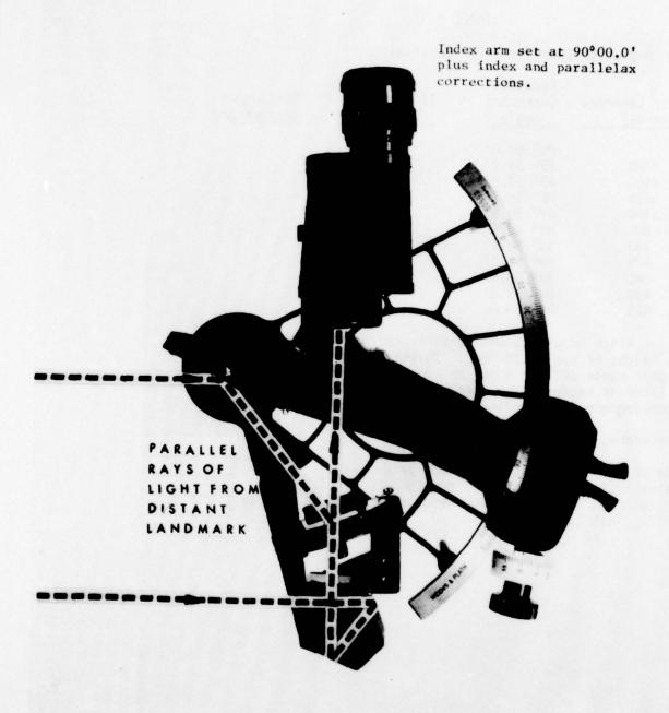
FIGURE 8. SURVEY SEXTANT WITH PENTA PRISM IN ADJUST POSITION. The light beams show how the penta prism subtracts 90°00.0' from the index arm reading when the penta prism is inserted with a counterclockwise turn.
