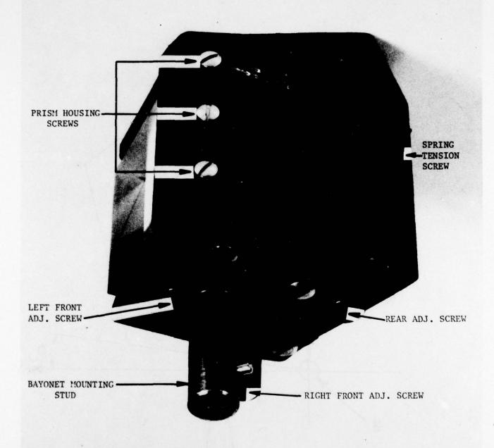
FIGURE 4. OBLIQUE VIEW OF PENTA PRISM SHOWING ADJUSTMENT SCREWS
