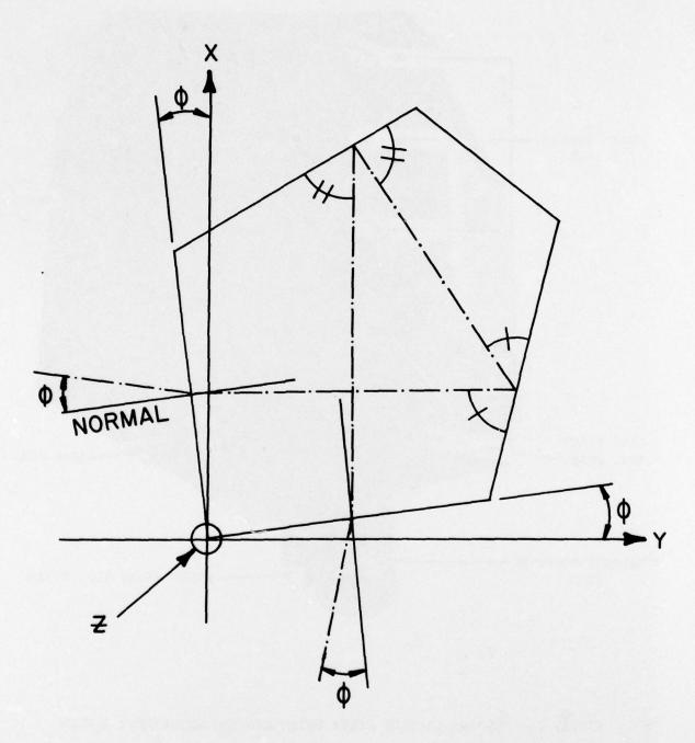
FIGURE 3. ROTATION ABOUT THE Z AXIS
