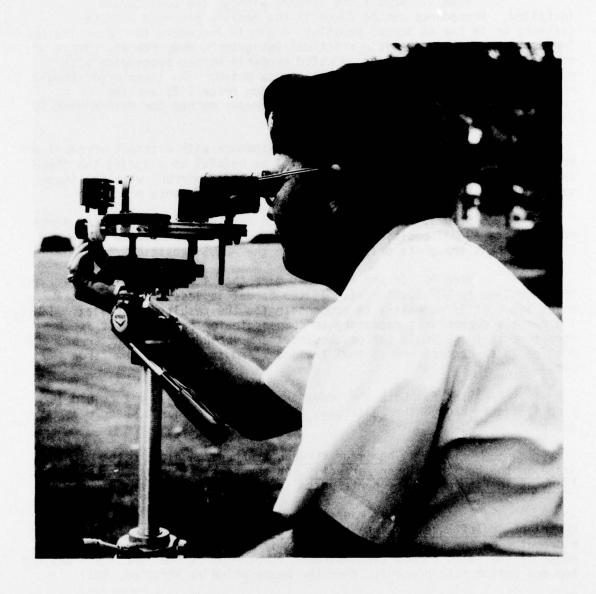
FIGURE 7. PENTA PRISM ADJUSTMENTS WITH SEXTANT MOUNTED ON A TRIPOD
