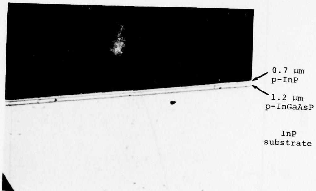
Fig. 51. Cleaved section of a hybrid heterojunction cathode.
