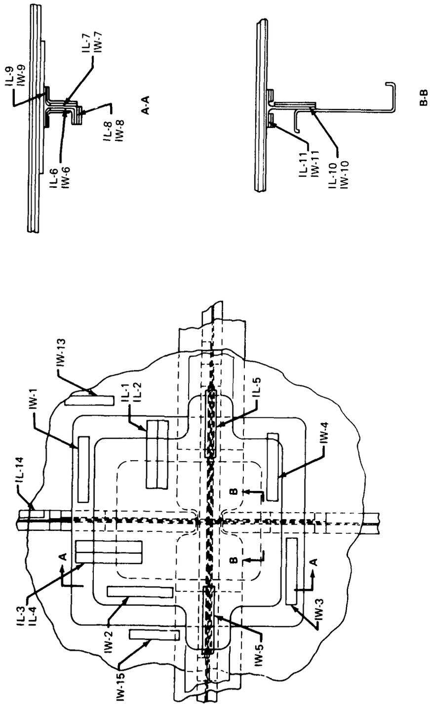
Figure 83.—Location of Specimens Cut from Internal Longeron Repair
