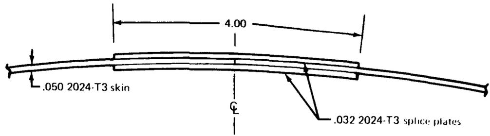
Figure 34. - Bonded Longitudinal Splice Detail - Pabst Baseline
