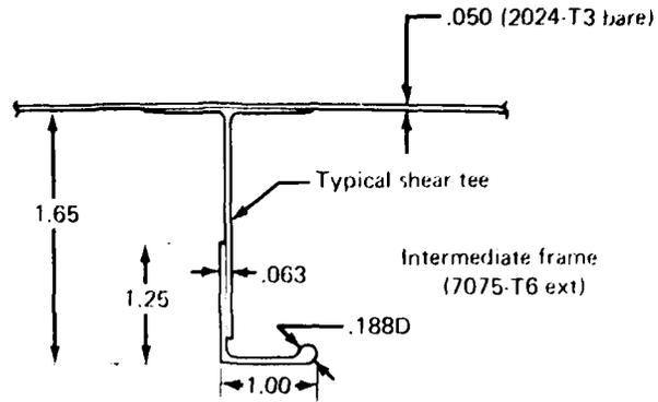
Figure 32. Typical Intermediate Frame Detail - Pabst Baseline
