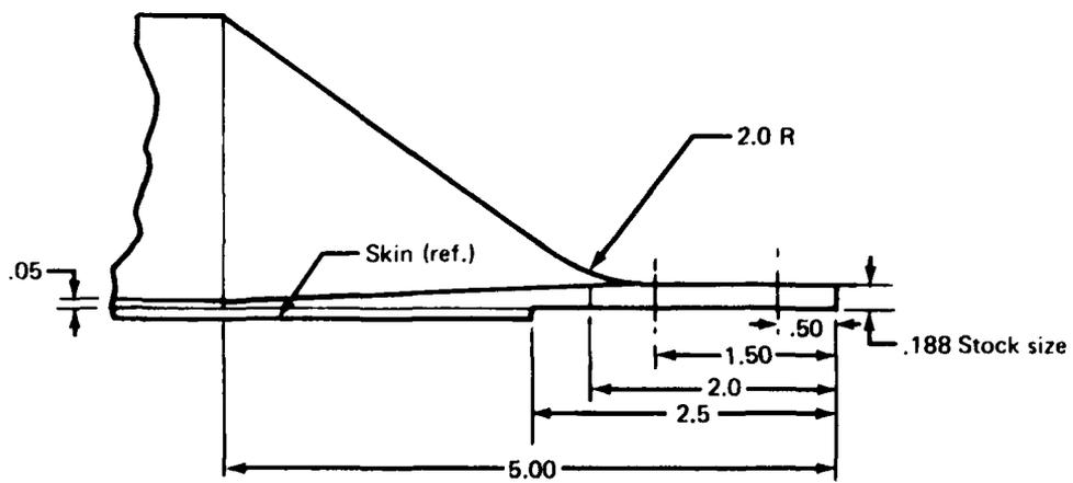
Figure 15.—Build-up Provided at End of Shear Panel Frame Tee for Test Loading.
