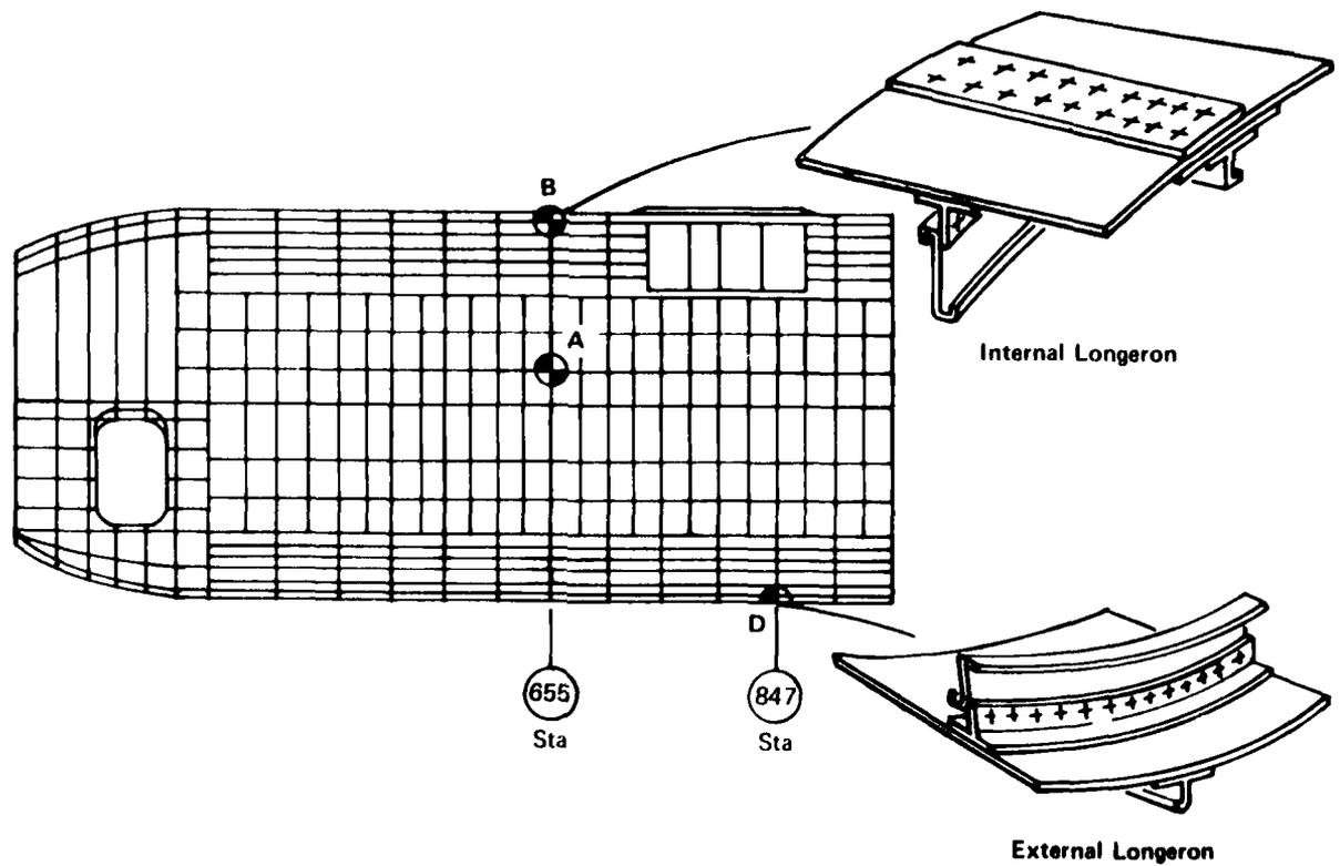
Figure 35. - Areas on Pabst Structure for Repair Study
