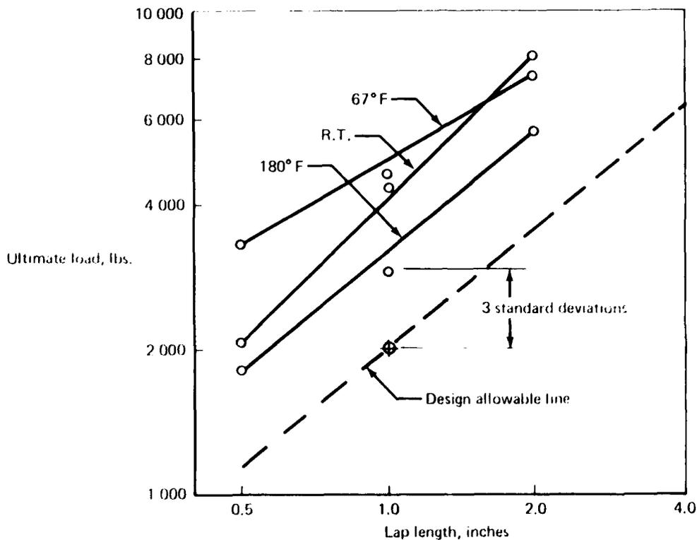
Figure 14. Design Curve Derivation - FM73 Adhesive
