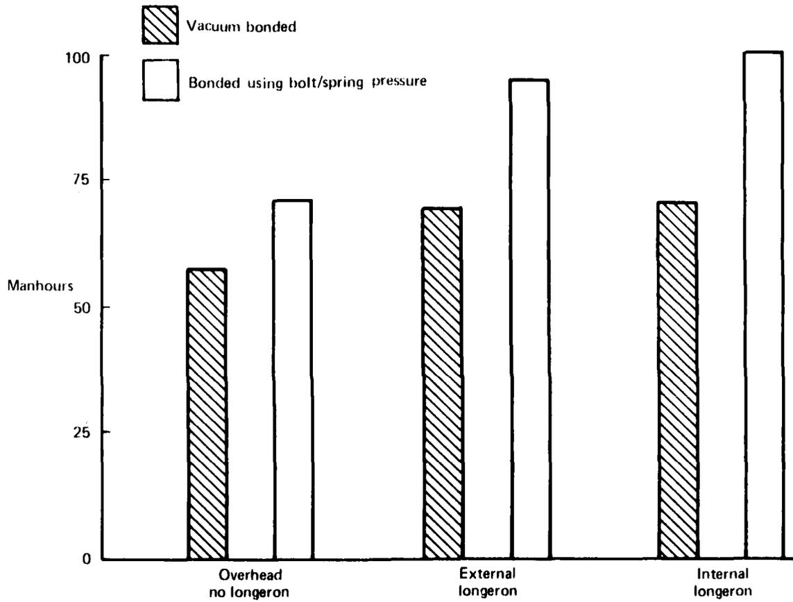
*Figure 92.—Comparative Man-hours Required for Repairs using Bolts/Springs for Pressure Application Versus Use of a Vacuum Bag*
