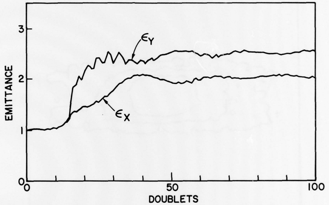
Fig. 4 - Evolution of the x-p_x and y-p_y rms emittances showing the establishment of a steady state.
