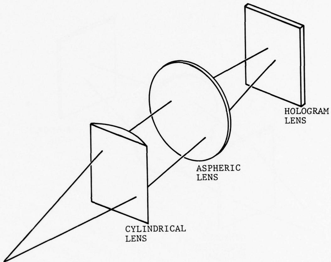
FIGURE 22. GENERATION OF ARBITRARY PHASE WAVEFRONT WITH CONVENTIONAL OPTICS
