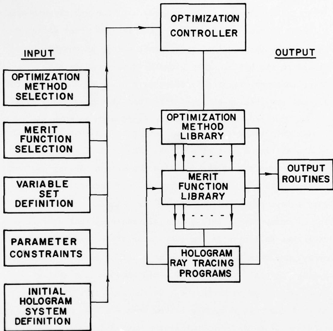
FIGURE 29. OPTIMIZATION PROGRAMS FOR HOLOGRAPHIC OPTICAL ELEMENTS
